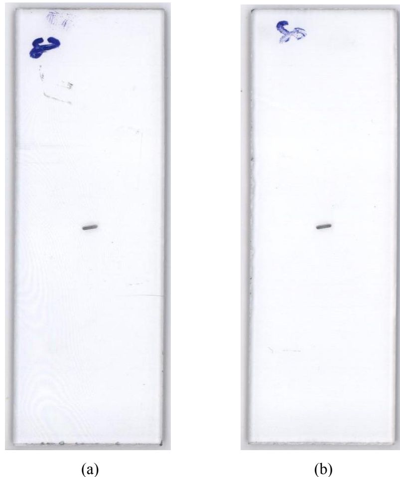
Figure 3.13. (a) PMMA specimens with an inclined crack, \beta = 80^\circ before tensile testing (b) PS specimens with an inclined crack, \beta = 80^\circ before tensile testing
