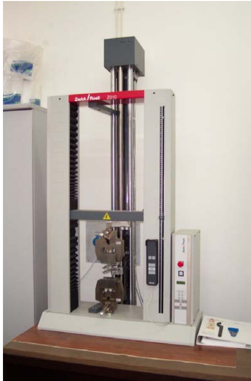
Figure 3.6. Zwick / Roell Z010 tensile testing machine
