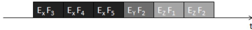
(a) Arriving sequence of the frames of the events ( E_i F_j stands for j^{th} frame of i^{th} event)
