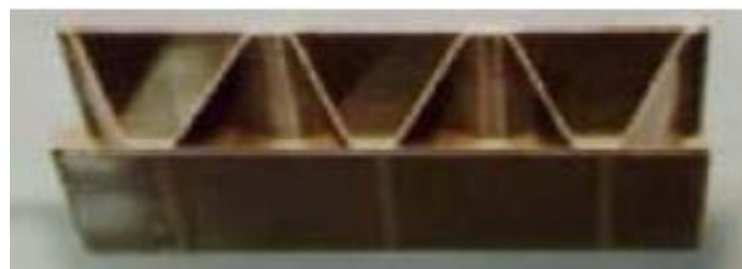
Figure 1.4. An industrial example of corrugated sandwich plate [9].
