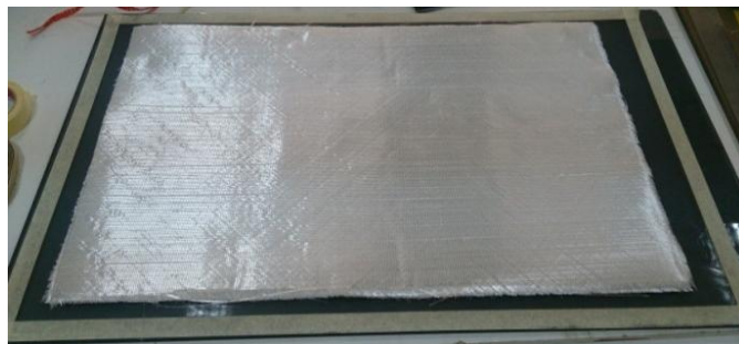
Figure 3.7. Placing of reinforcements on the glass surface.
