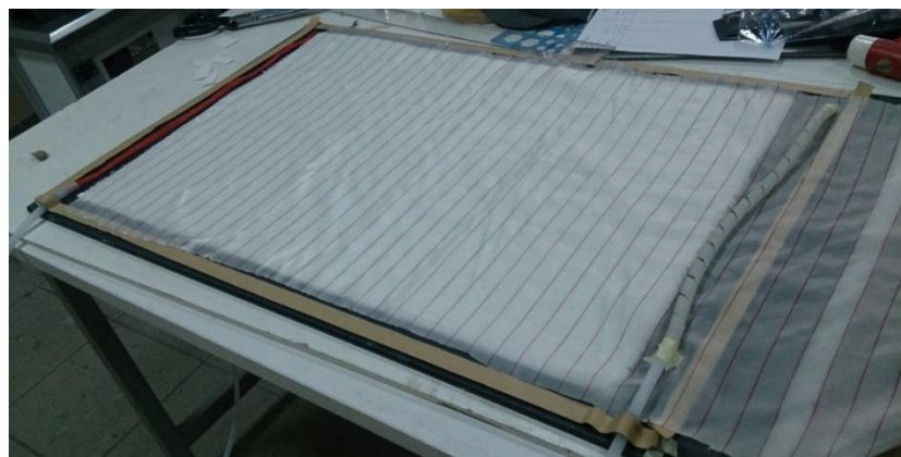
Figure 3.9. Placement of peel ply.
