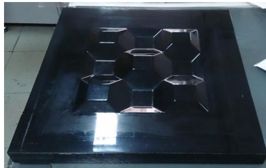
Figure 3.2. The lacquer coated mold.
