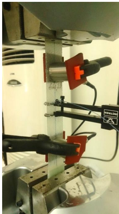
Figure 5.2. Installation of piezoelectric transducers.
