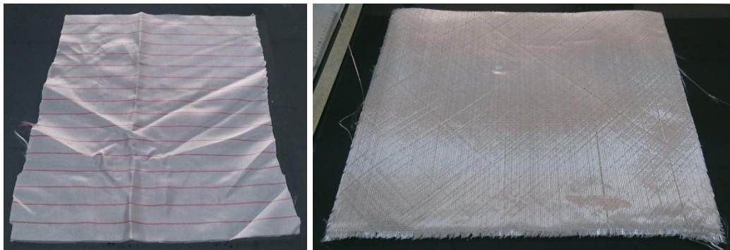
Figure 3.3. (a) Peel ply and (b) glass-fiber reinforcement.
