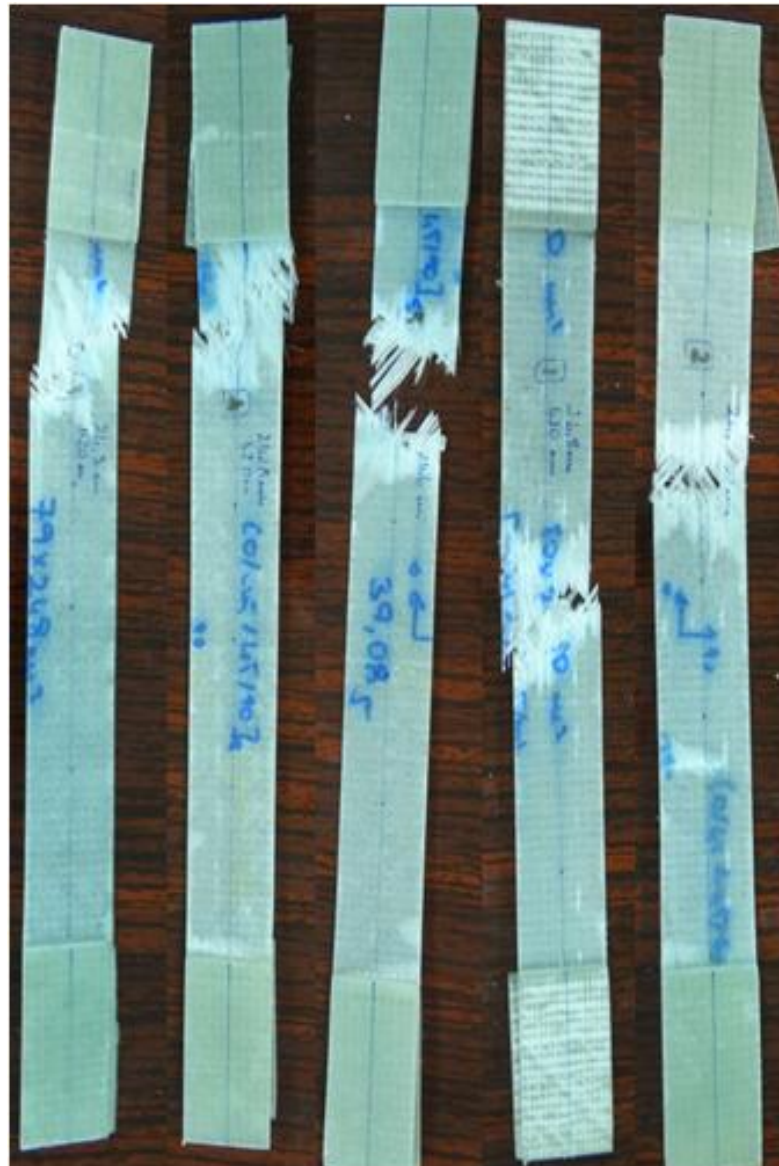
Figure 5.4. Failed quasi-isotropic specimens.
