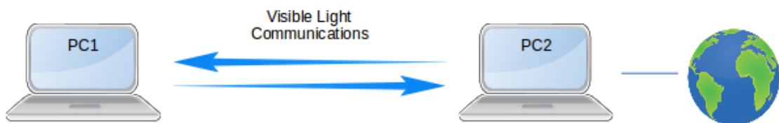
Figure 1.1. Simple Li-Fi System
