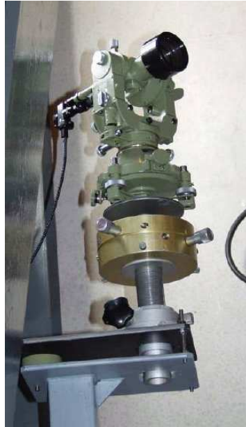
Figure 6.11. Photograph of the theodolite employed for the alignment
