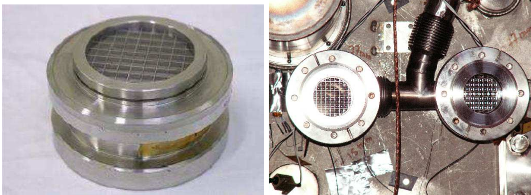
Figure 4.4. The cold windows, outside of the magnet and mounted on the cold bore. The gas input/output lines can also be seen in the right picture
