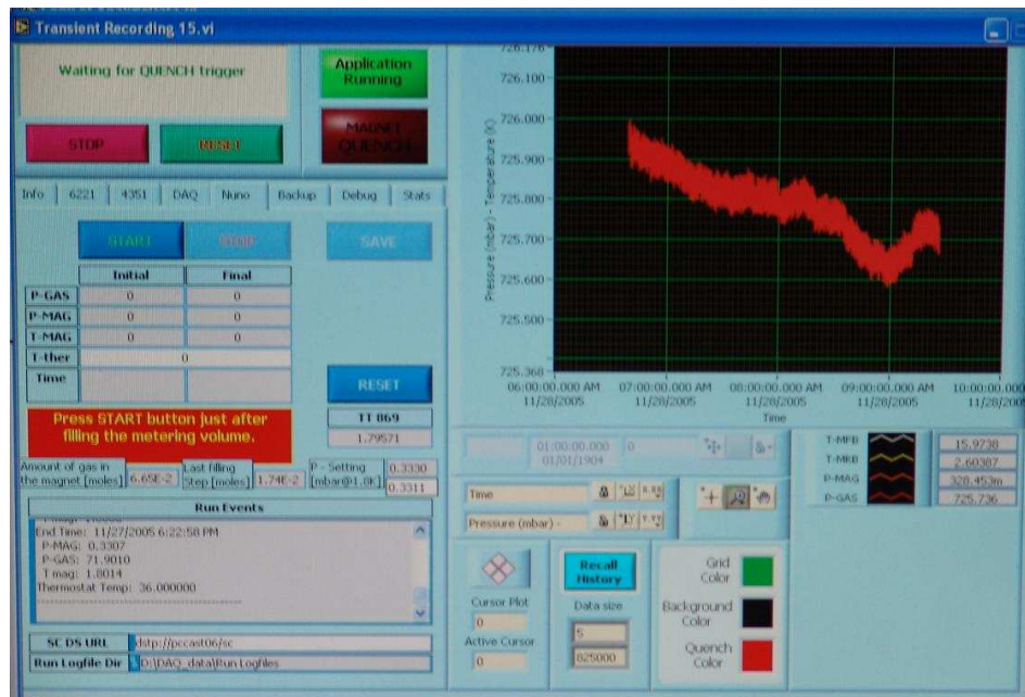
Figure 5.6. The transient recording program, which monitors the ^4\text{He} pressure and the temperature, among other things. The picture doesn't show the displayed metering volume pressure, which wasn't implemented at the time of this screenshot
