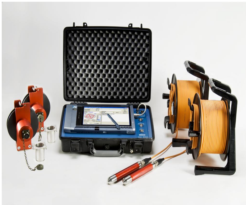
Figure 5.37. The cross hole ultrasonic monitor system ( http://www.piletest.com )
