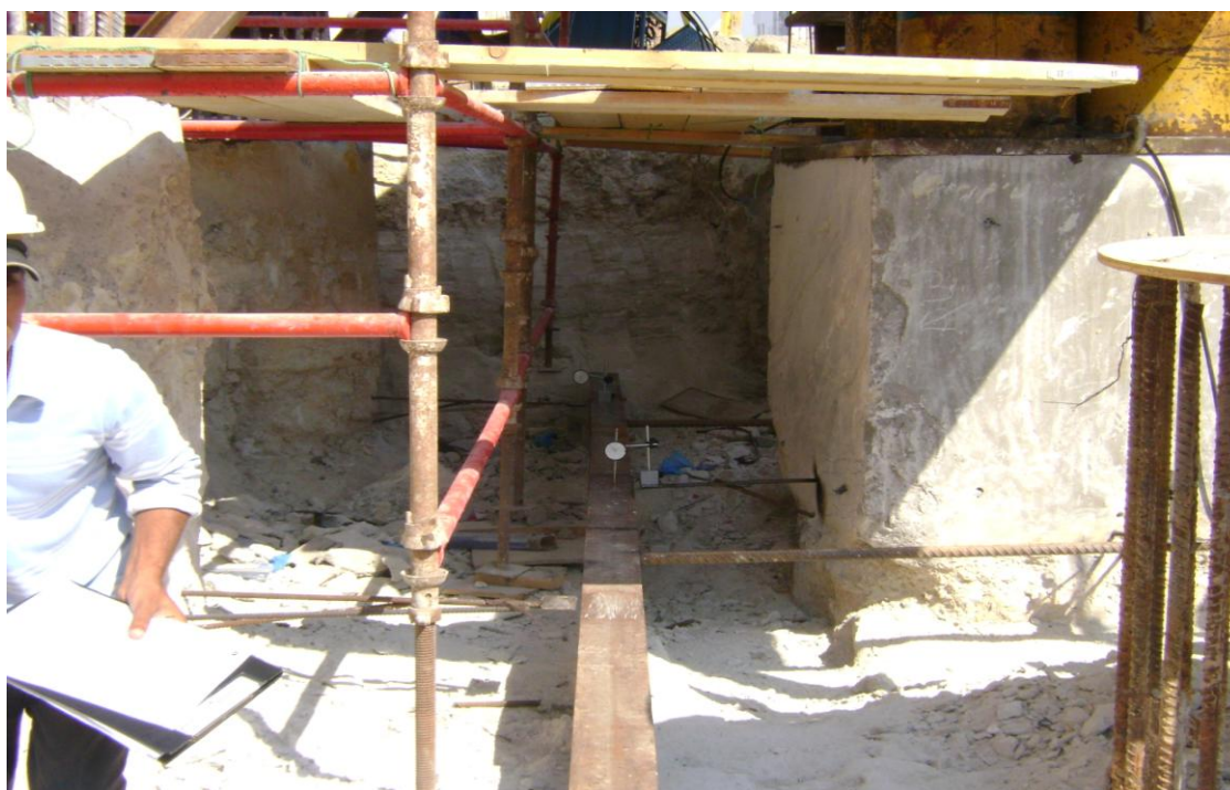
Figure 6.11. Micrometers used for displacement readings
