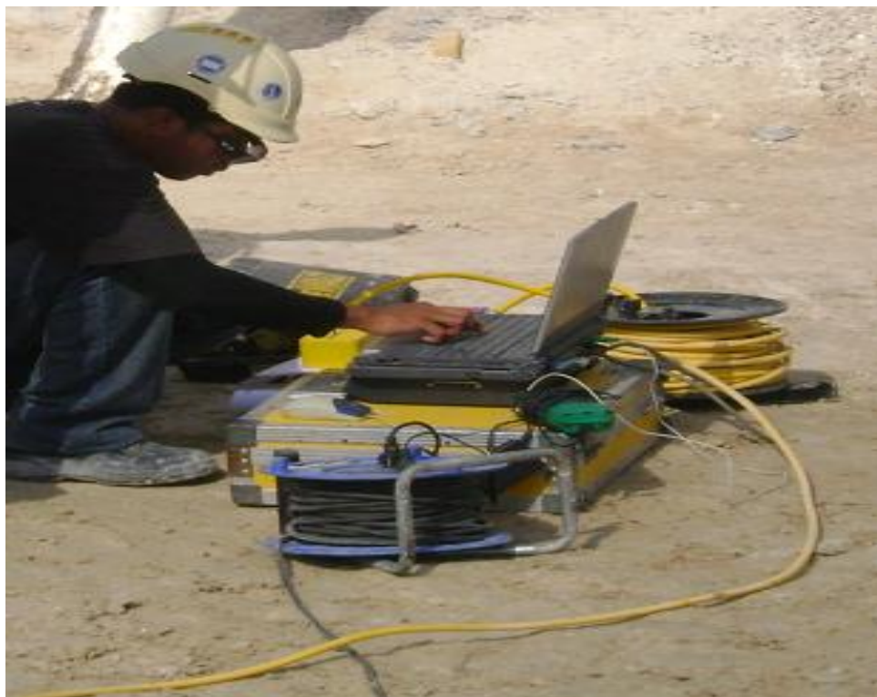
Figure 5.32. Pile driving analyser on field
