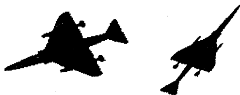
Figure 4.5. The reference image of an object and an affine transformed version
