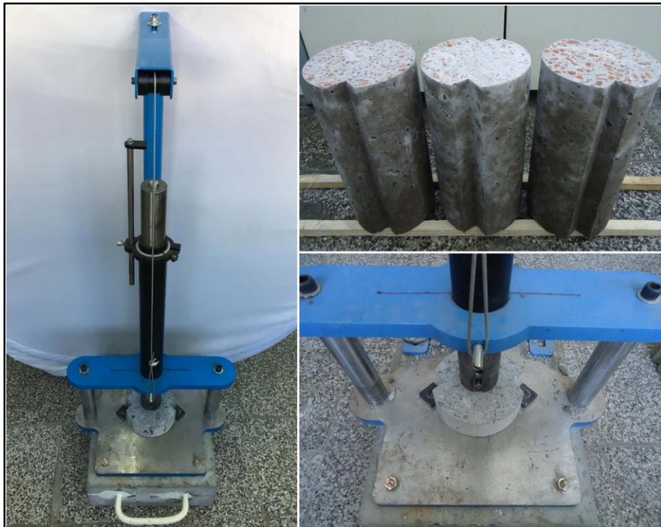
Figure 3.10. Test setup for drop weight impact resistance.
