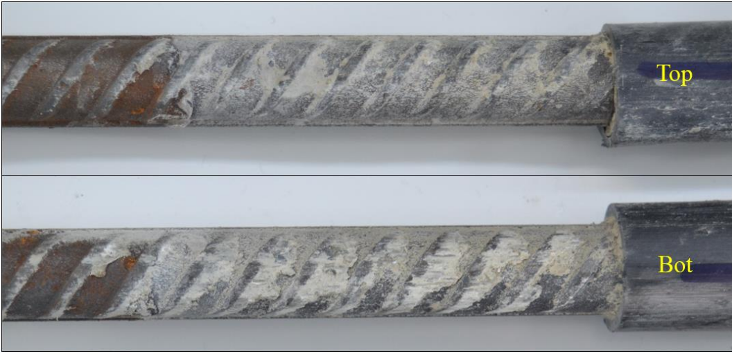
Figure 4.37. Mortar adhered on bars in a column specimen of TRCAC.
