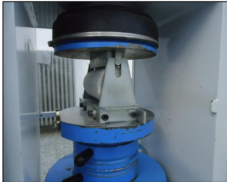
Figure 3.8. Test setup for splitting tensile strength.
