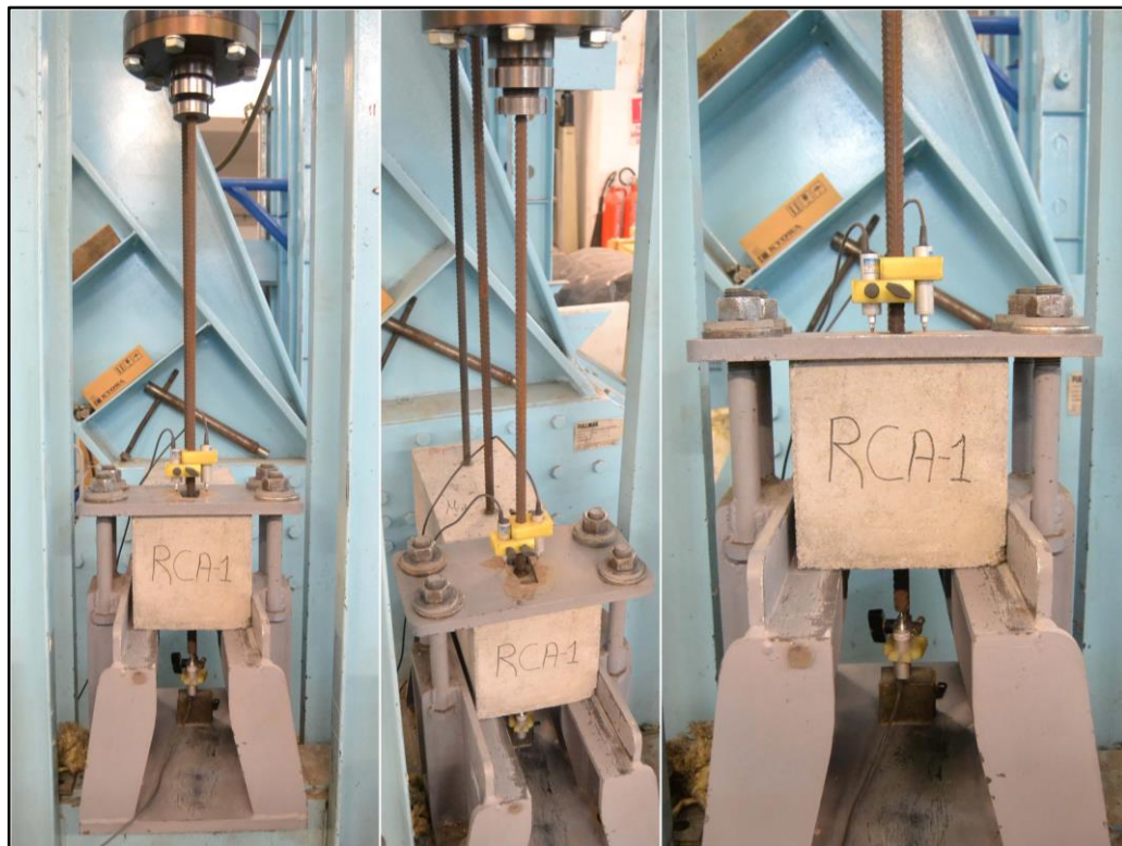
Figure 3.16. Test setup for pull-out test on column specimens.
