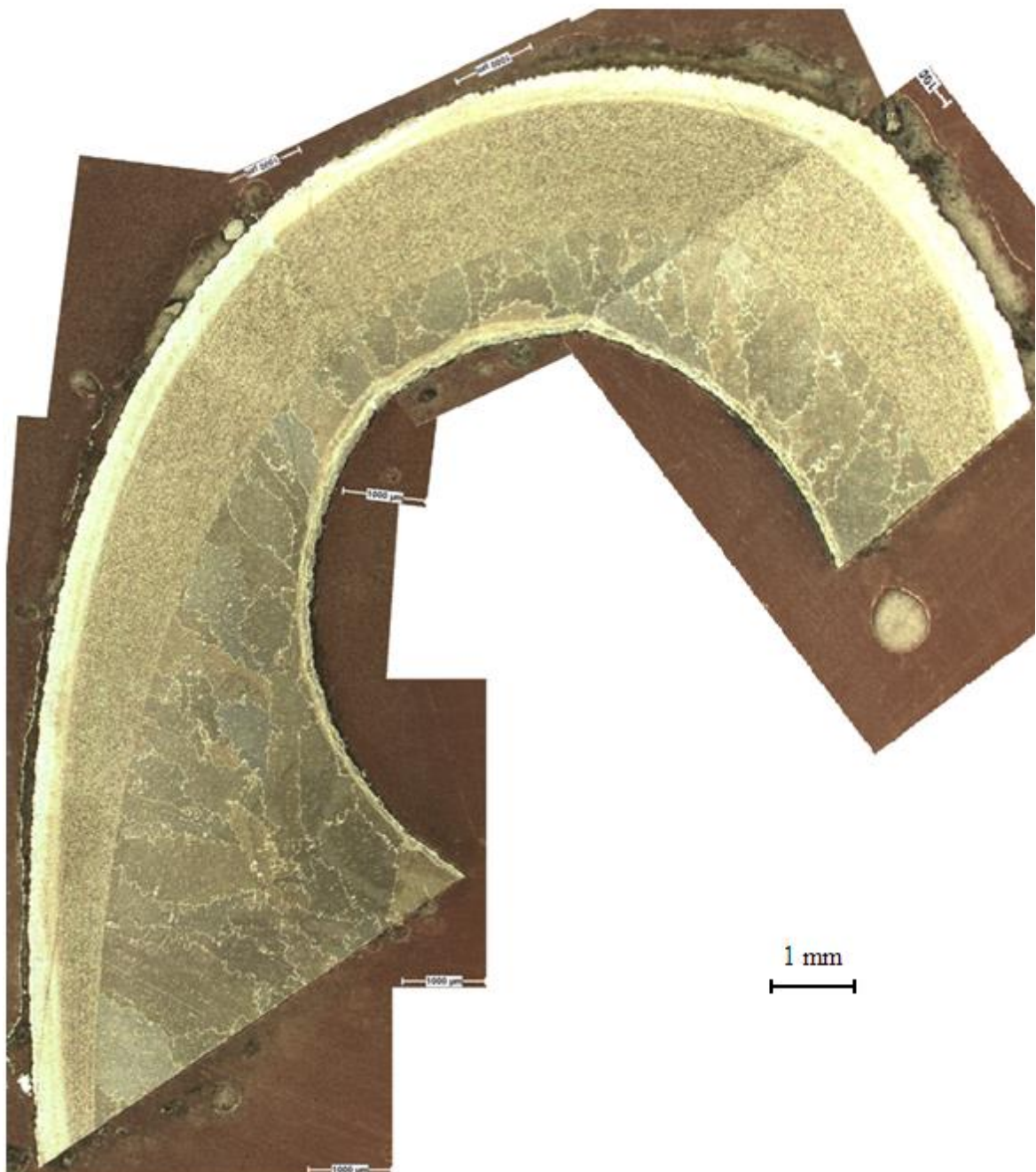
Figure 3.3. Coatings in SPO-TL (tip section, leading edge) position.
