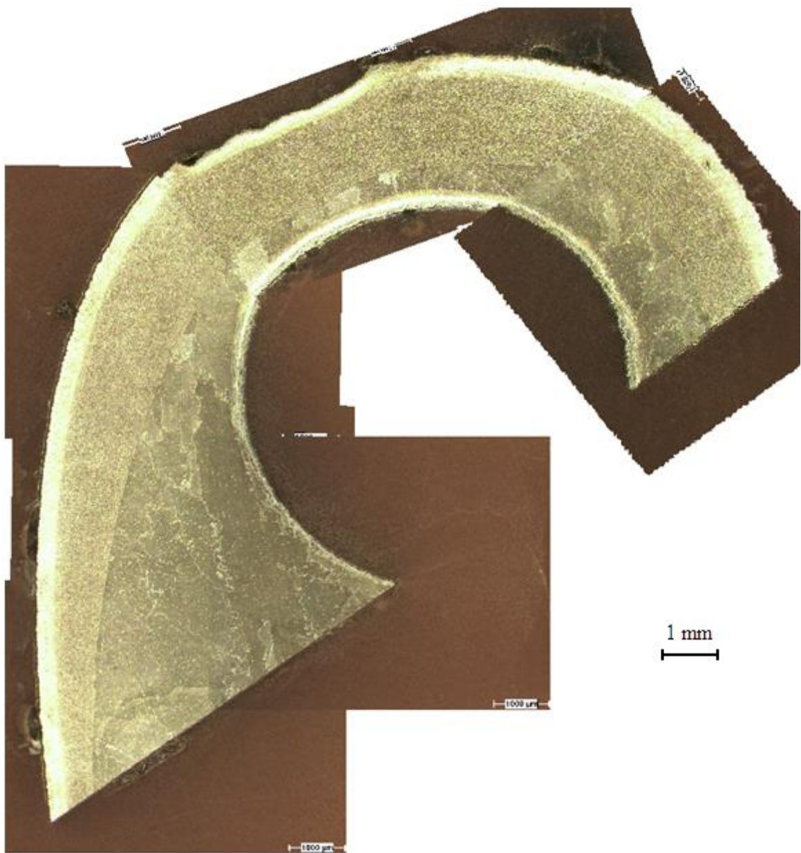
Figure 3.4. Coatings in SPO-ML (middle section, leading edge) position.
