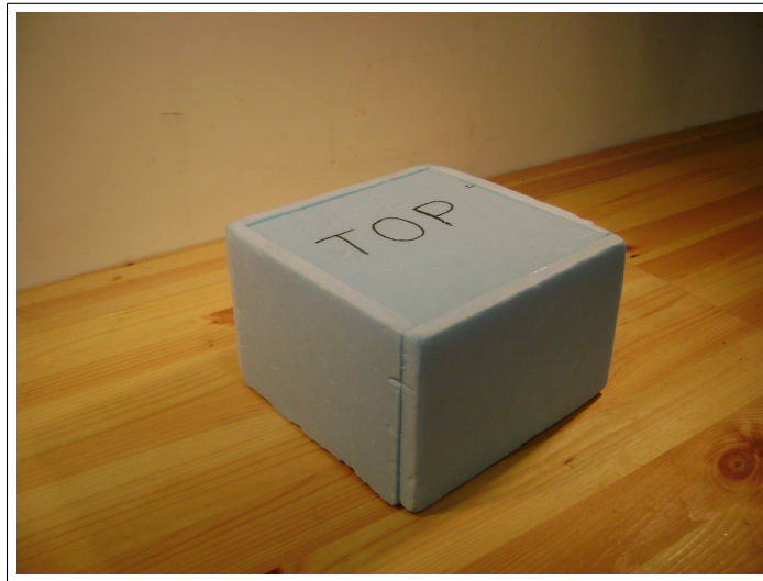
Figure 4.1 Rectangular gel phantom with heat insulation
