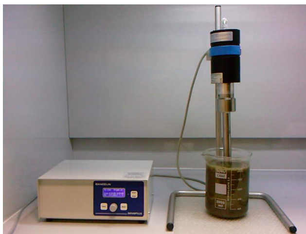
Figure 3.1. The ultrasonic homogenizer used in the study (Bandelin-Sonopuls HD 3400).
