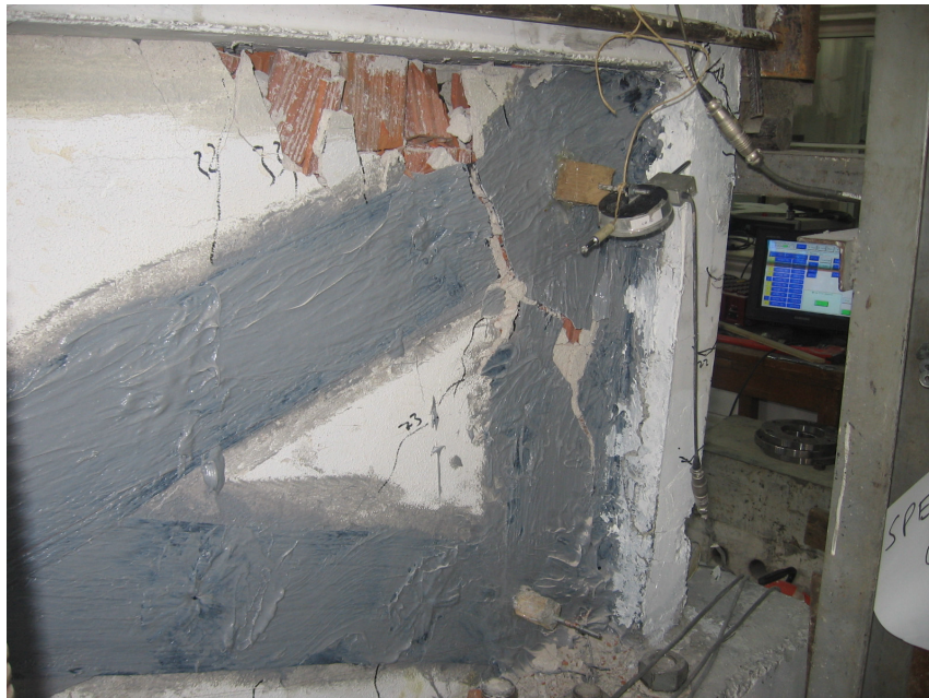
Figure 4.15. Rupturing of diagonal and vertical FRP for front side of specimen O2
