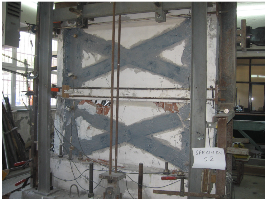
Figure 4.17. Condition of specimen O2 after the test
