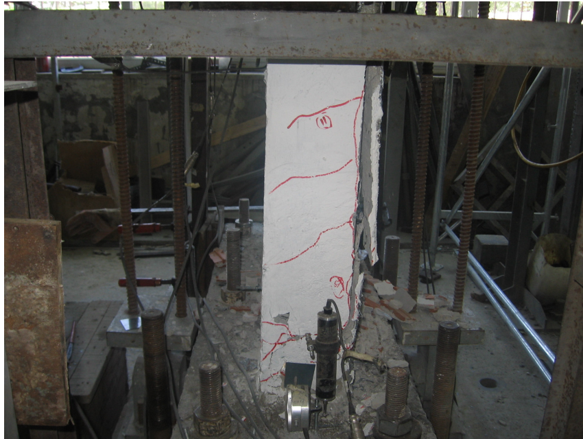
Figure 4.7. Tension cracks on right column of specimen O1
