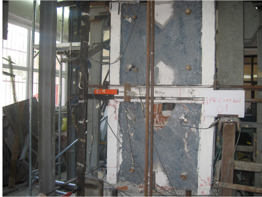
Figure 4.9. Condition of specimen O1 after the test
