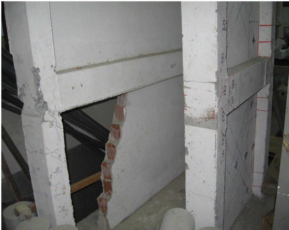
Figure 3.4. First floor of test specimens
