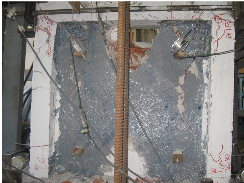
Figure 4.6. Final condition of frontside of specimen O1
