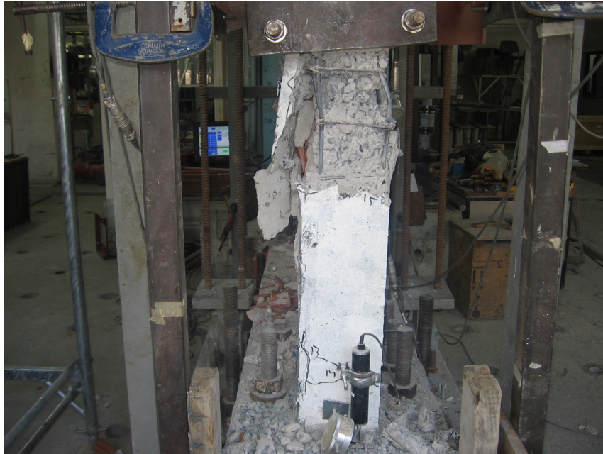
Figure 4.16. Spalling of concrete and buckling of reinforcement
