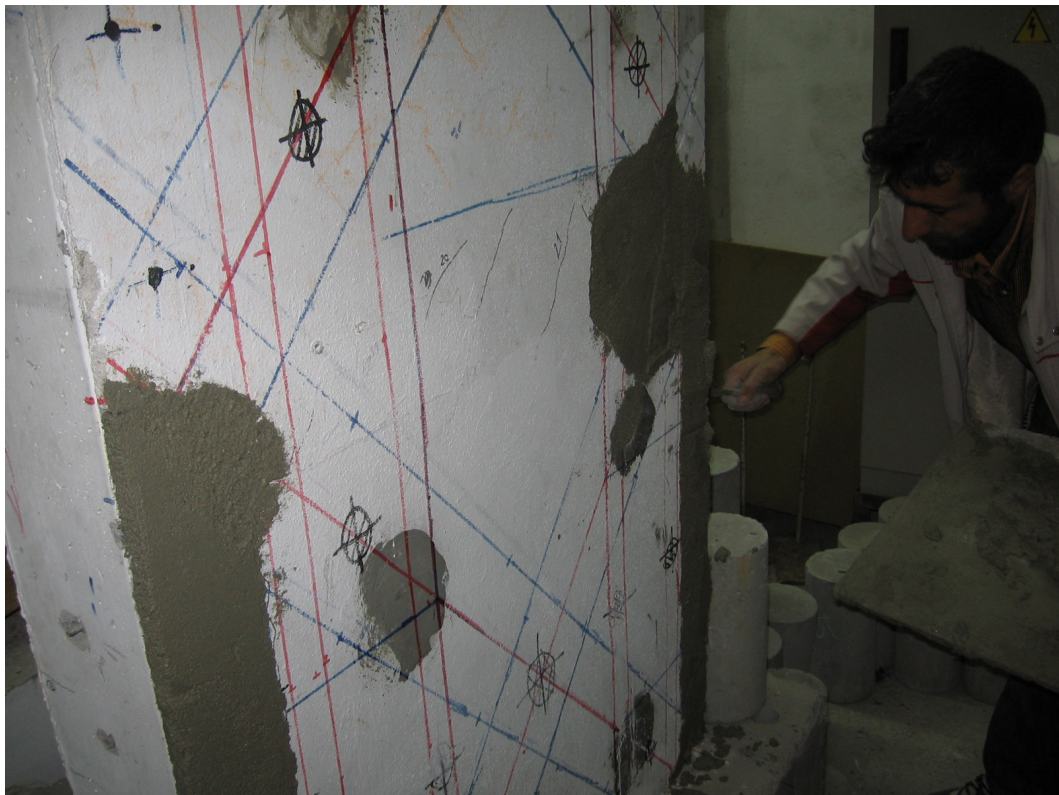
Figure 3.8. Plaster repairs for specimen O1
