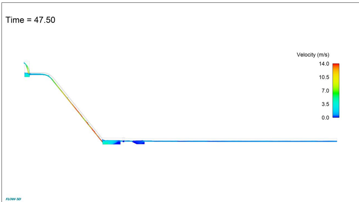
Figure 4.30. Flow 3D Velocity Distribution Along the Whole System (2D View at the Center of the Channel and Pools)
