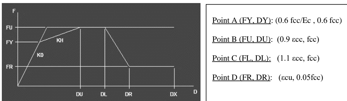
Figure A.1. Unconfined concrete stress-strain relationship, Perform 3D idealization points.
