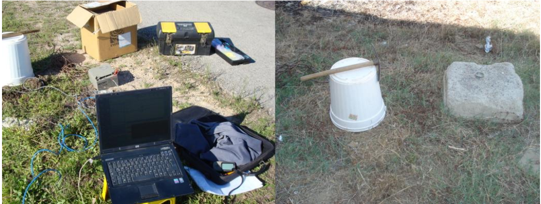
Figure 6.2. Left figure shows seismic equipment in one measurement point. Right one shows seismometer installation next to a borehole to decrease effects of wind, a bucket was put on the seismometer
