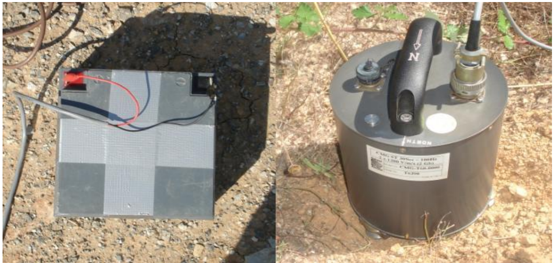
Figure 6.3. Left figure shows power supply, Right figure shows GÜRALP CMG-6T seismometer
