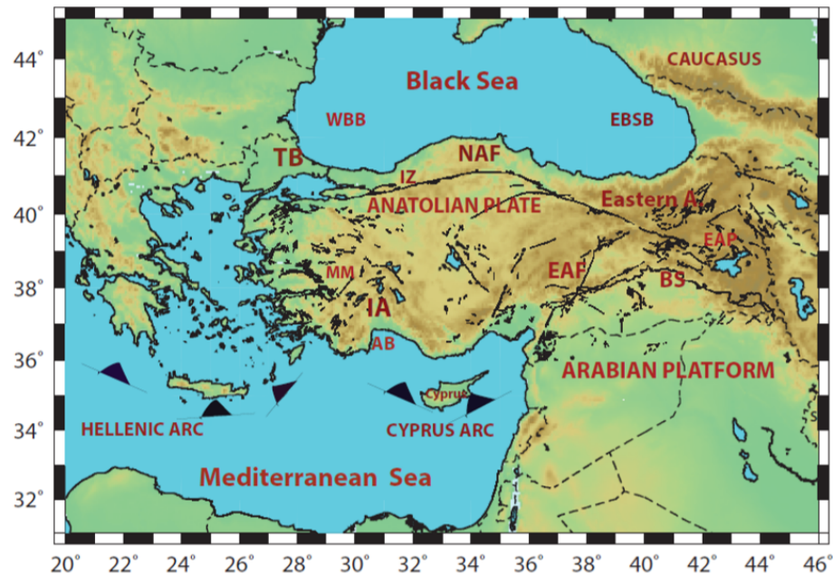
Figure 2.1. A simplified tectonic map of Turkey and surroundings. (AB) Antalya Basin; (BS) Bitlis Suture; (EAF) East Anatolian Fault; (EAP) Eastern Anatolia Plateau; (EBSB) Eastern Black Sea Basin; (IA) Isparta Angle; (HA) Hellenic Arc; (CA) Cyrus Arc; (IZ) Istanbul Zone; (MM) Menderes Massif; (NAF) North Anatolian Fault; (TB) Thrace Basin; and (WBB) Western Black Sea Basin.
