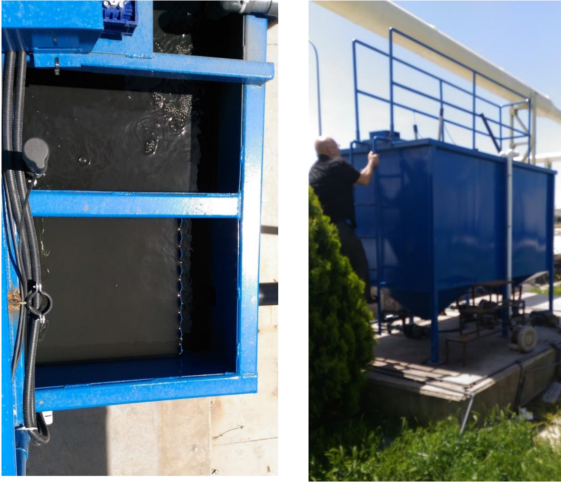
Figure 3.17. Pilot plant of Biofilm Nitrification - Contact Denitrification System.
