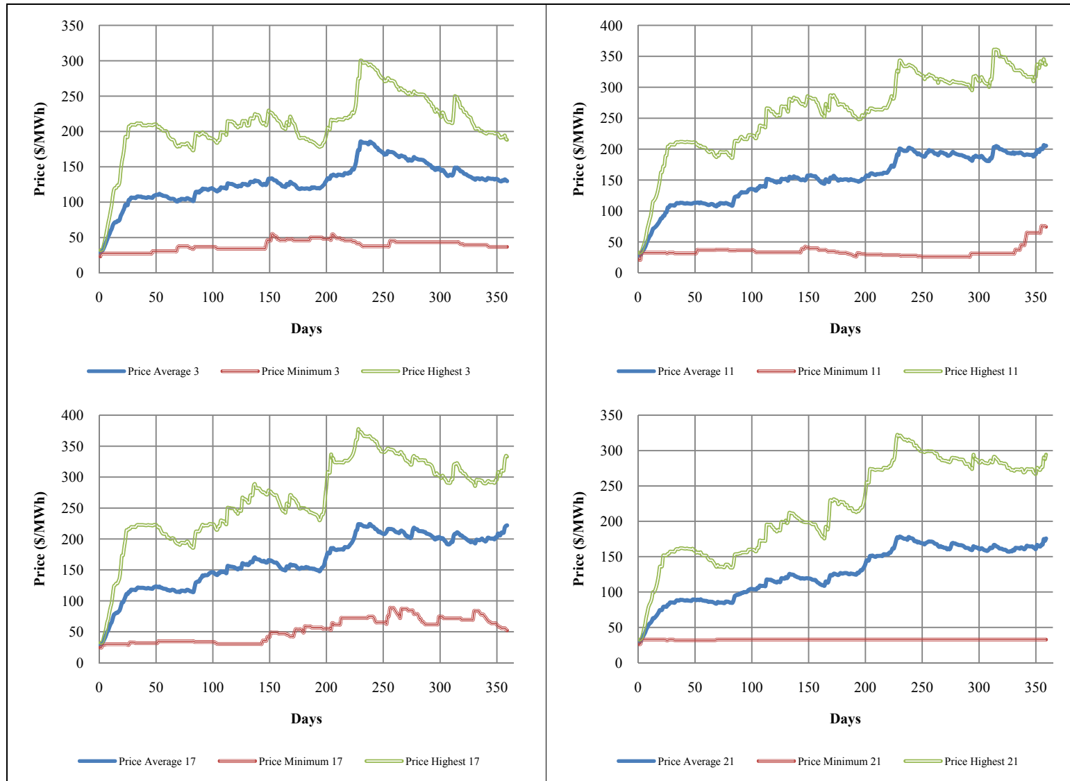
Figure 4.39. Impacts of high transmission fee scenario on electricity sales prices at the selected time intervals (AC OPF case).
