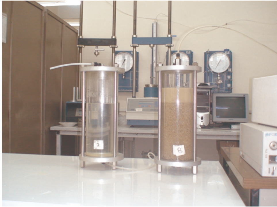
Figure 3.4. Bentonite injection in sand test set up.
