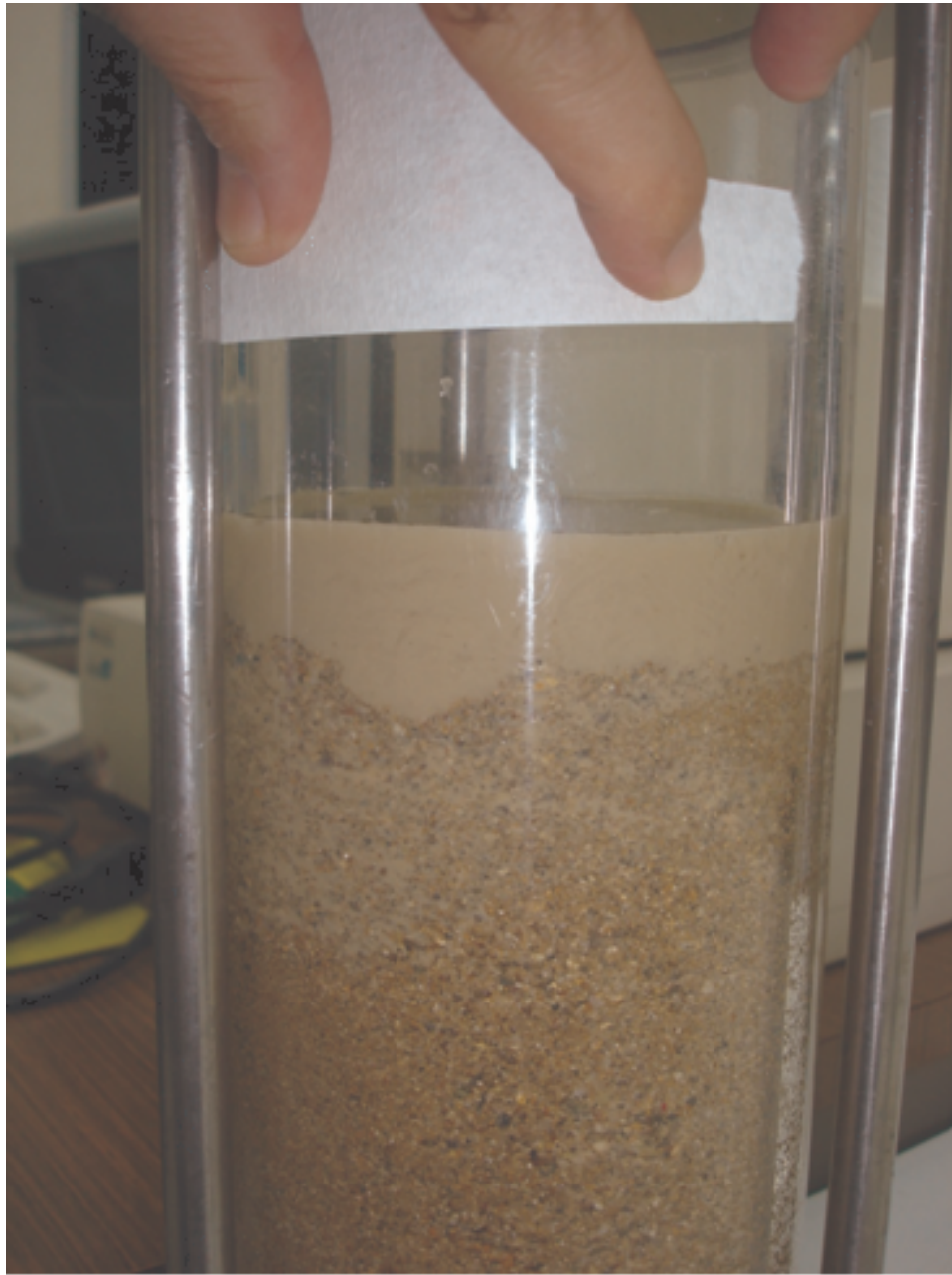
Figure 3.9. 5% Bentonite injection just after preparation.
