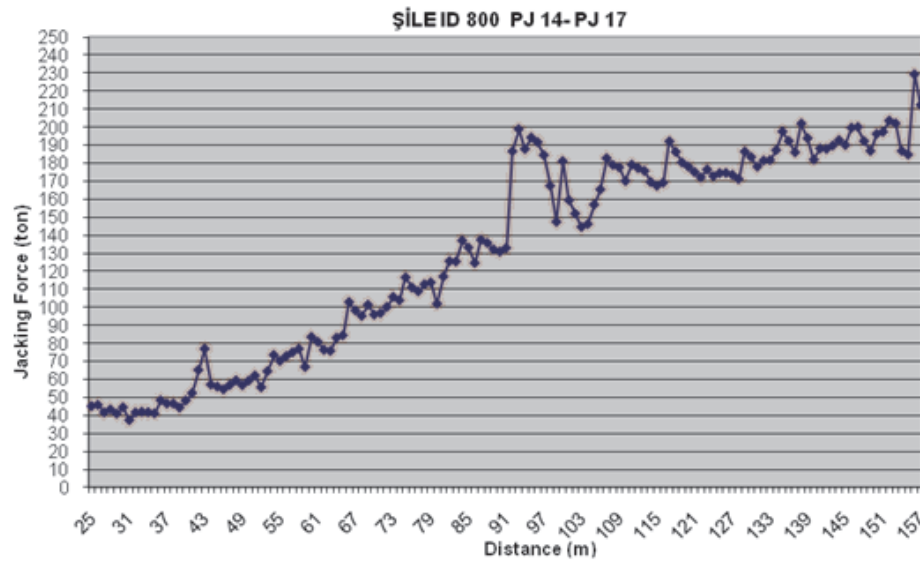
Figure 4.4. Collector project pipe jacking data between pits 14-17.
