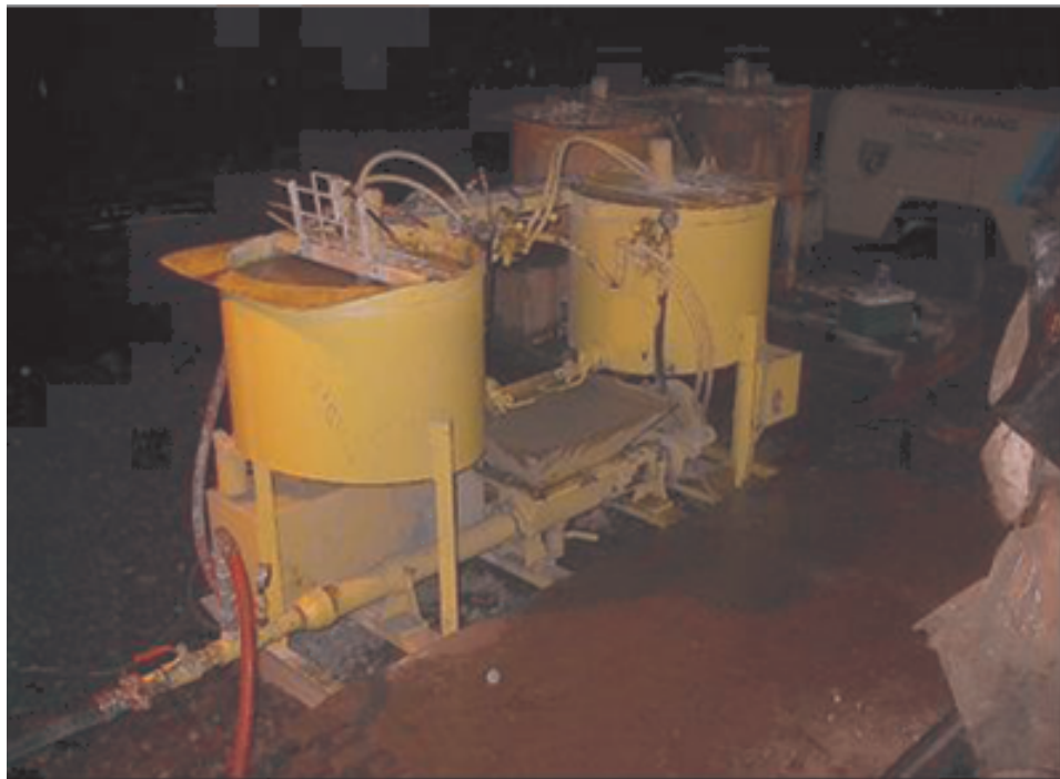
Figure 3.1. Controlled injection of bentonite (Staheli, 2006).
