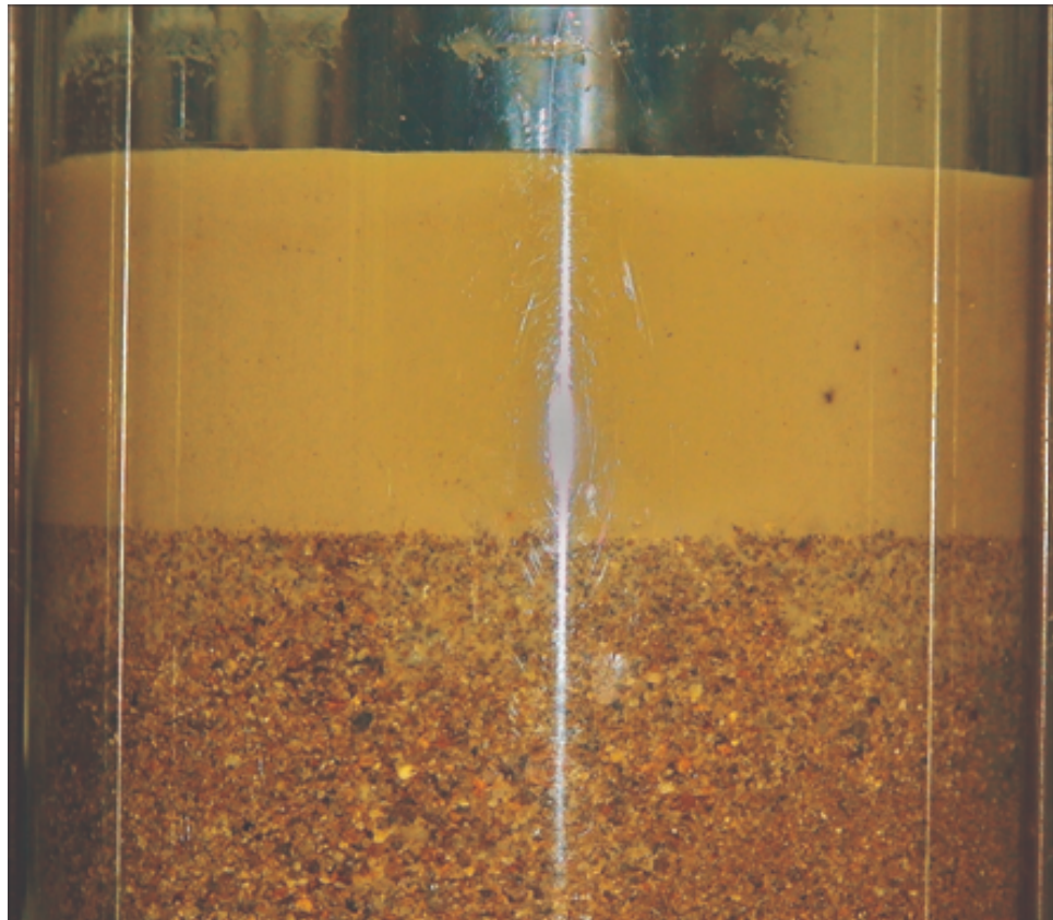
Figure 3.8. 6% Bentonite injection after 24 hours of hydration.
