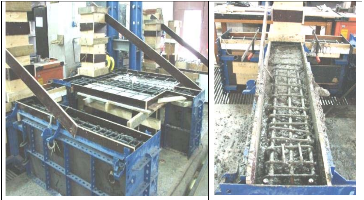
Figure 3.24. Construction of specimens
