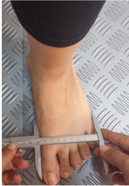
Figure 4.15. Measurement of foot breadth obtained by caliper.
