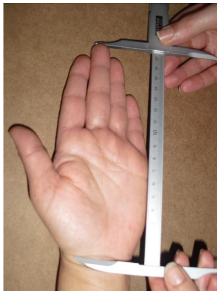
Figure 4.16. Measurement of hand length obtained by caliper.
