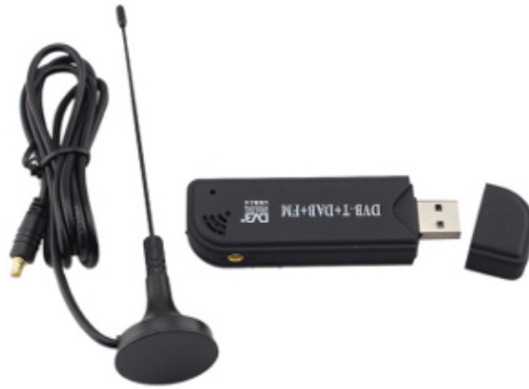
Figure 3.2. DVB-T receiver dongle and its antenna.
