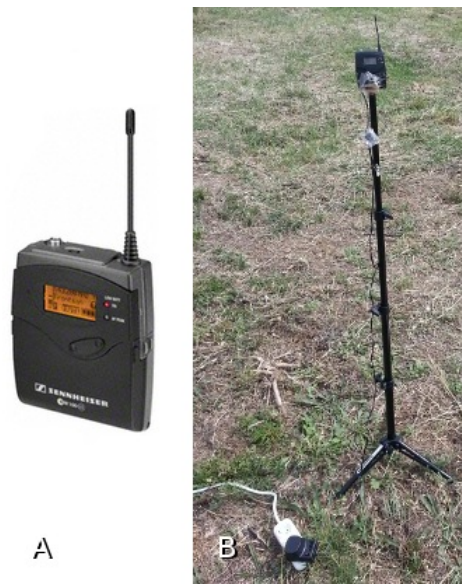
Figure 3.1. The transmitter powered with an external adapter on a tripod.
