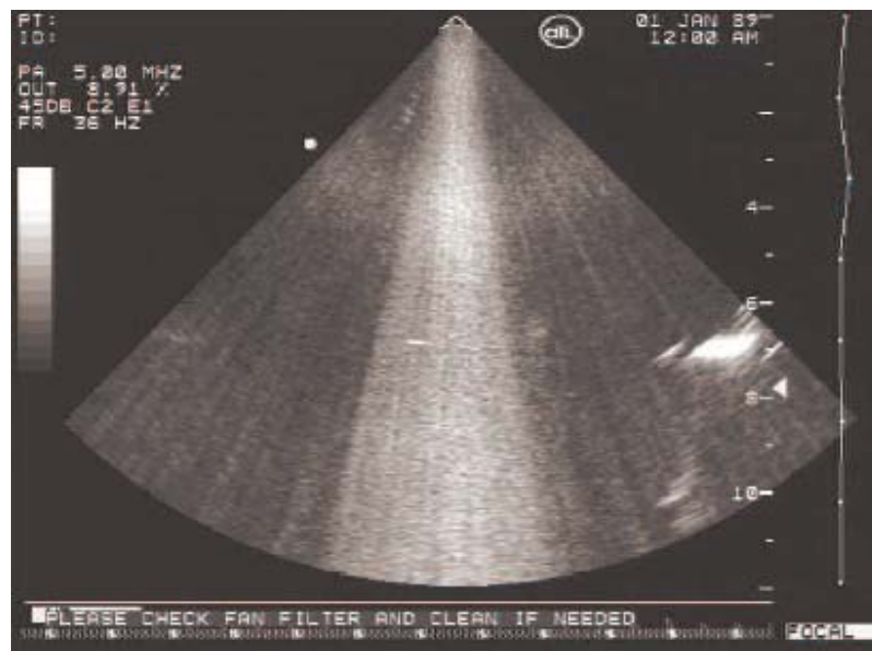
Figure 4.1 Visualization of the interaction between the HIFU transducer and the US scanner.
