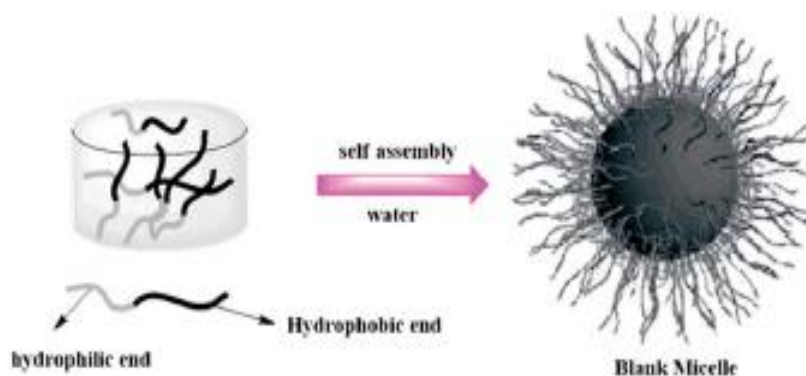
Figure 1.13. Schematic illustration of polymer micelle formation. Amphiphilic copolymers self-assemble to have a hydrophobic core and a hydrophilic corona structure in aqueous environments [21].
