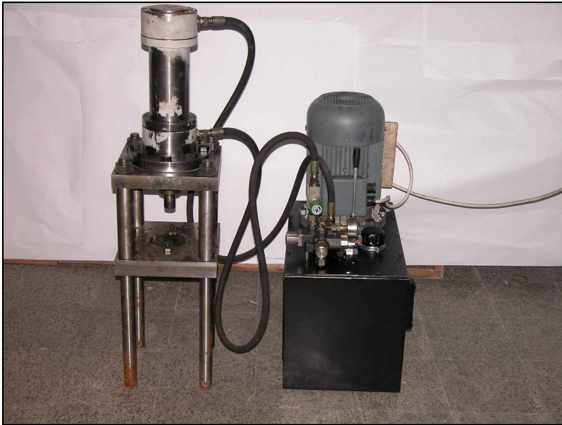
Figure 5.13. Semi-solid forming unit
