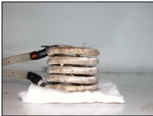
Figure 5.7. The photo and specifications of the heating coil
