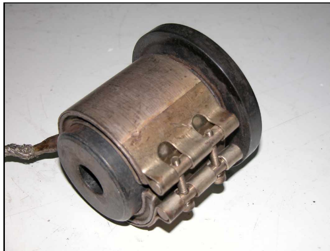
Figure 5.12. The ring heater in combination with the main part of the die
