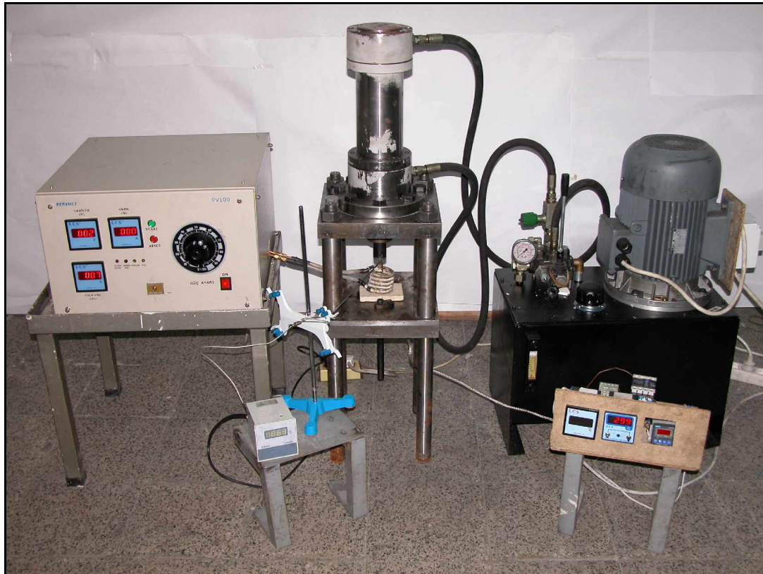
Figure 5.17. An appearance of thixoforming system in operation
