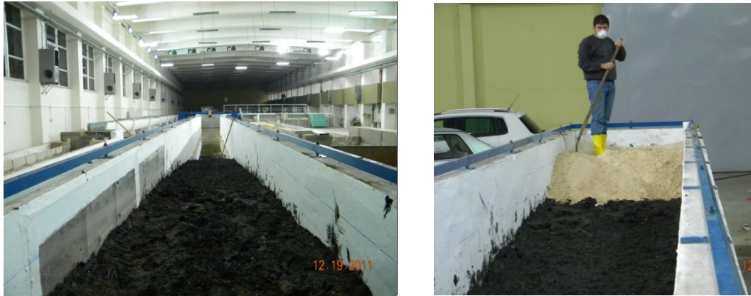
Figure 4.7. Placement of the model materials into the wave channel.
