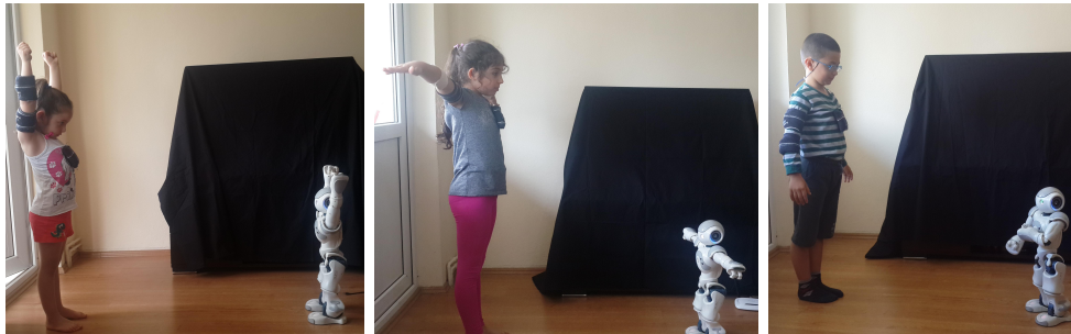
Figure 6.16. Lower arm sensor positioning caused wrong make elbow straight feedback
