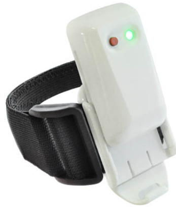
Figure 4.8. EXL-S3 Wireless Inertial Measurement Unit
