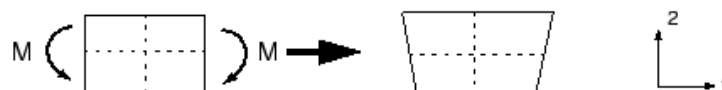
Figure 4.9. Deformation of a linear element with reduced integration subjected to bending moment M [56].
