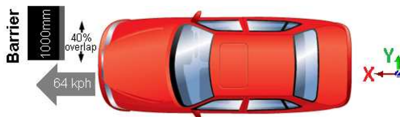
Figure 2.1. A scheme for EuroNCAP Frontal offset crash tests [42].
