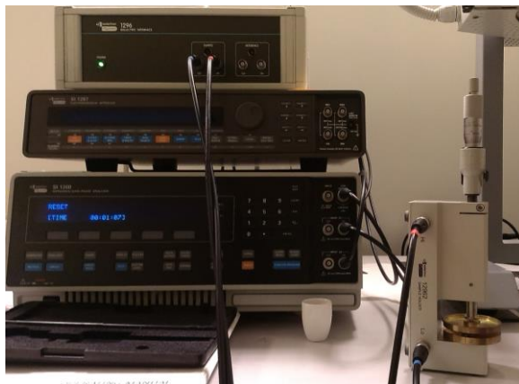
Figure 2.18. Solartron analytical 1260 impedance/Gain device and placement of the silver-coated sample between two cylindrical copper parts.
