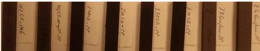
Figure 2.19. Grinded samples ready to be silver coated.
