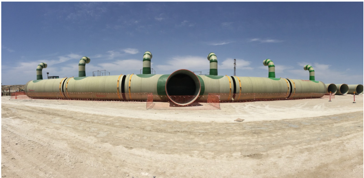
Figure 4.11. Photograph of the diffuser. Photograph is taken from Murat Cenk Gerdanlı - MCG Mühendislik.
