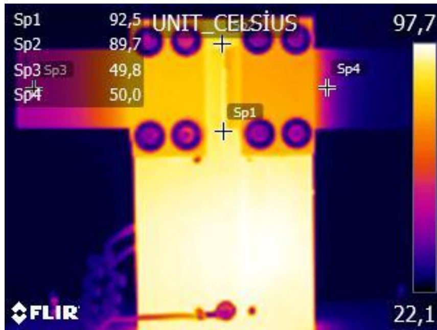
Figure 4.54. Thermal Camera View of Standard Stainless Steel Part (on the left) vs. 10% by Weight Carbon Fiber Filled Surlyn®1601 Composite Part (on the right).
