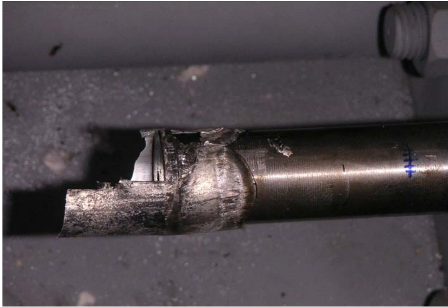
Figure 5.16. Reverse-coating of aluminum over the ram during the extrusion
