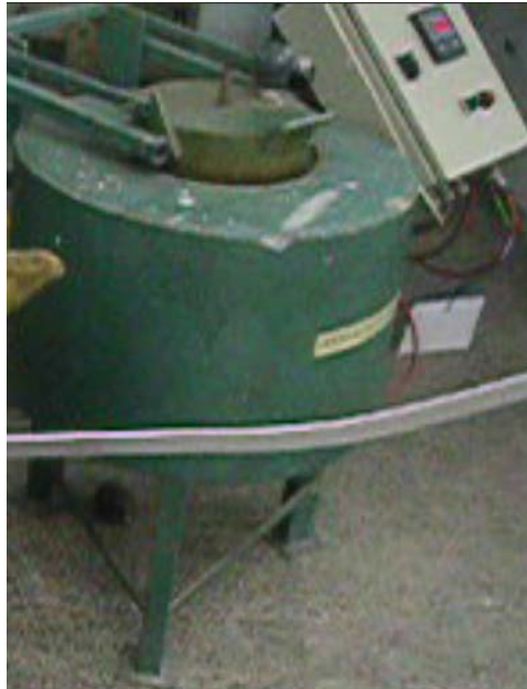
Figure 5.13. Furnace used to heat billet, container and die set
