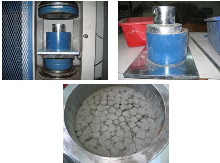
Figure 4.7. Aggregate crushing value test
