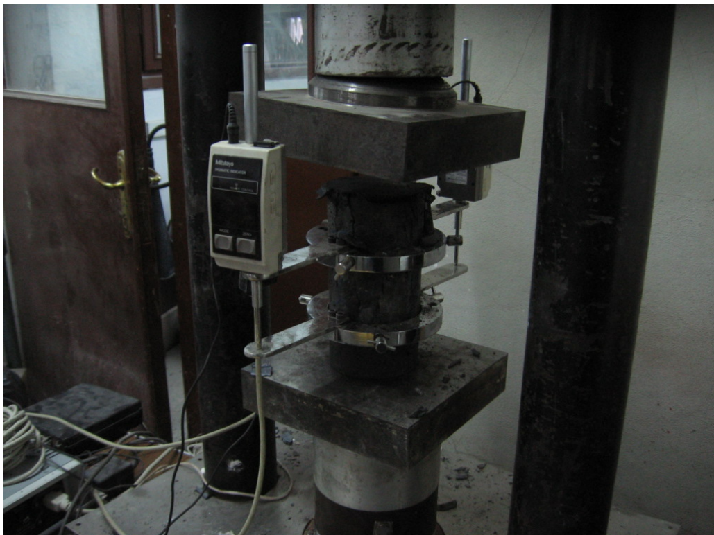
Figure 5.97. The view of concrete specimen after compression test
