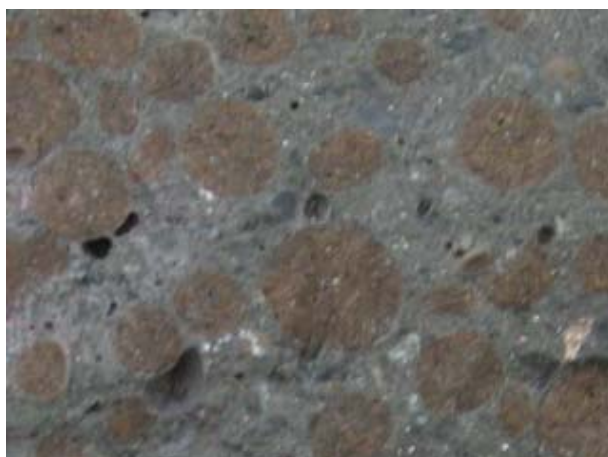
Figure 5.27. The fragments of crushed 10B1200 pellets in the fractured concrete
