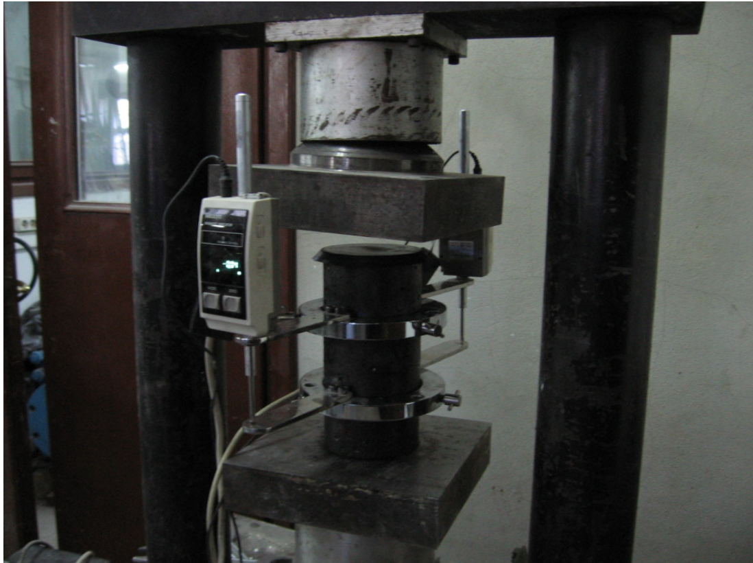
Figure 4.8. Compressive strength and modulus of elasticity test of hardened concrete
