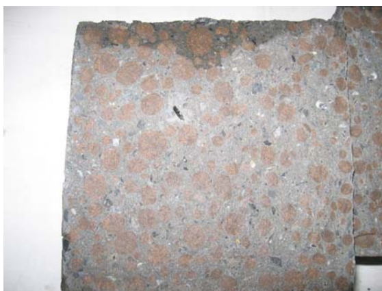
Figure 5.121. Determination of water penetration depth on splitted cubic specimen
