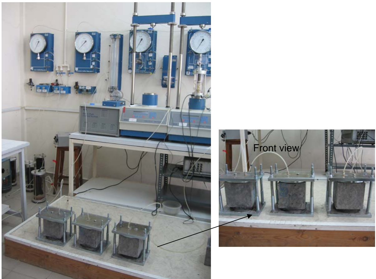
Figure 4.11. Water impermeability test
