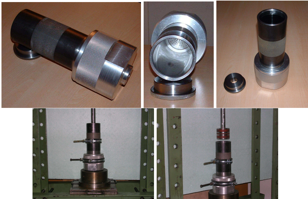
Figure 6.1. Aluminium pressure slip casting set-up
