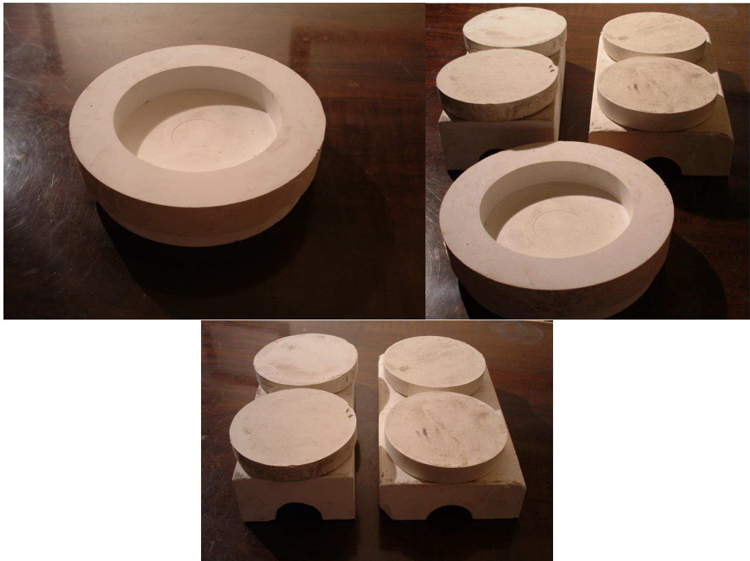
Figure 6.4. The ceramic pressure slip casting molds, shaped in plaster of paris mold
