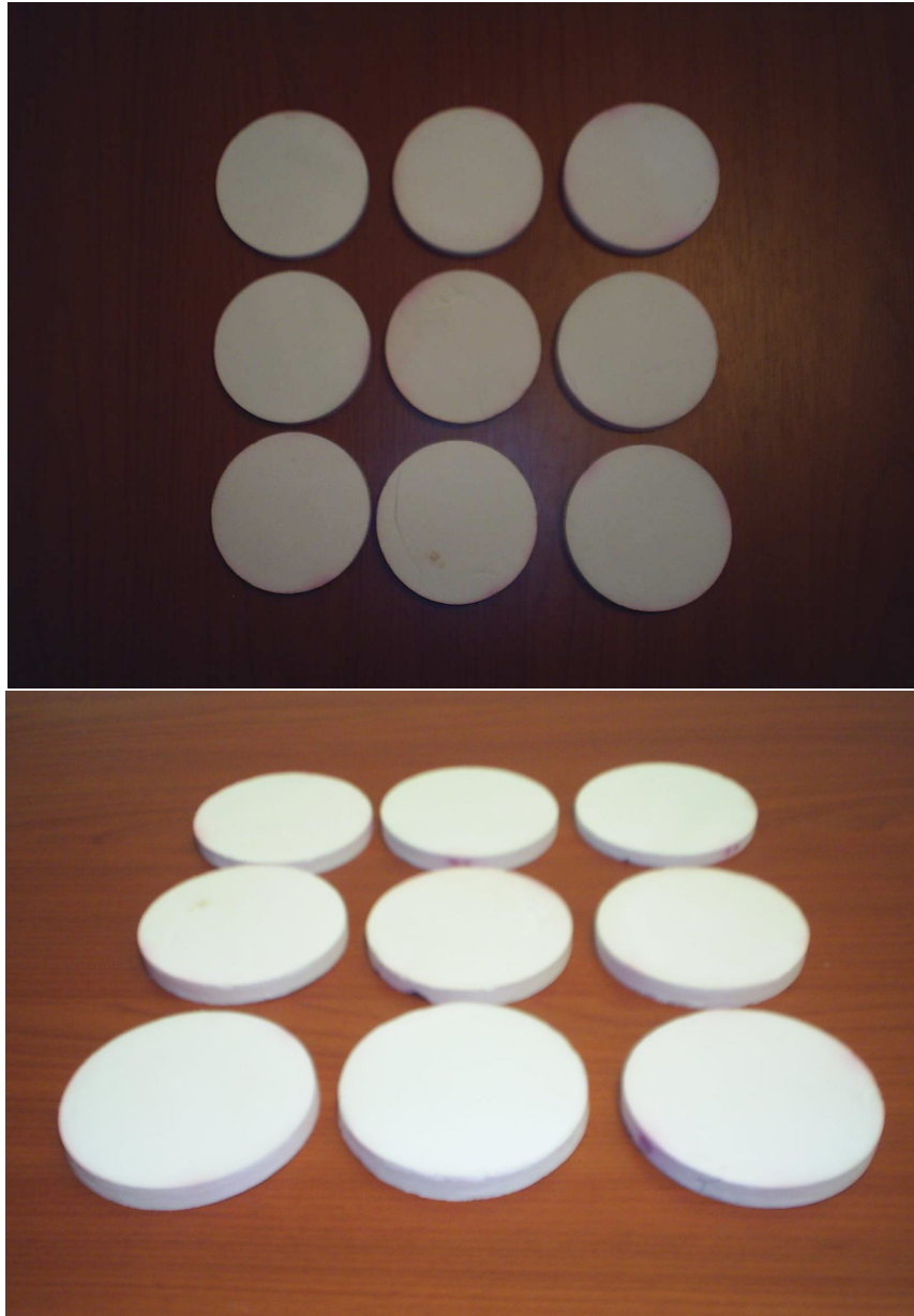
Figure 6.5. The produced cylindrical alumina ceramic compact parts
