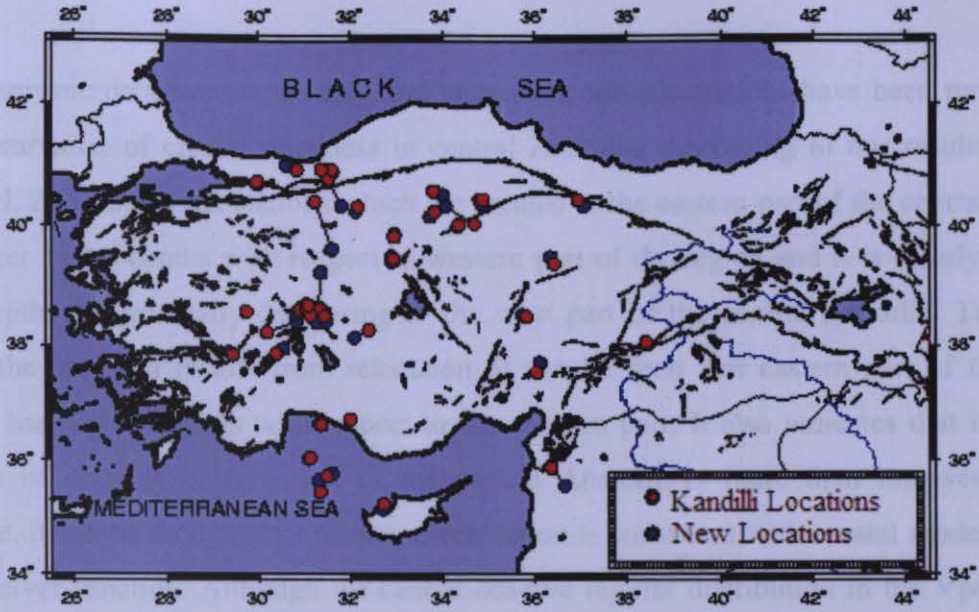
Figure 4.4 Difference between Kandilli locations and new locations calculated from second velocity model.
