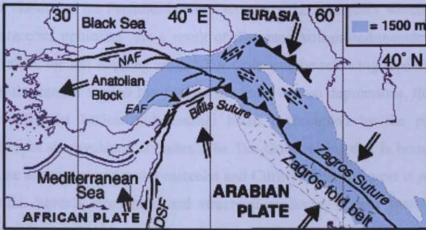
Figure 1.2 Map showing major tectonic structures of Turkey and adjacent areas. (modified after Şeber et al., 1997)
