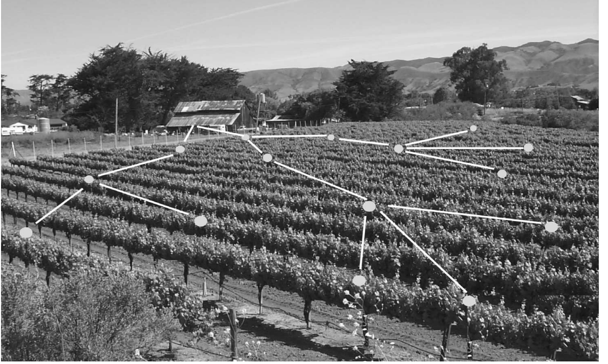
Figure 1.1. A WSN which collects temperature and moisture data
