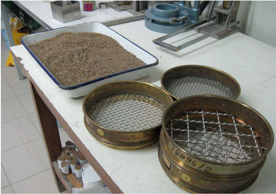
Figure 5.11. Various sizes of sieves used in preparing greywacke samples
