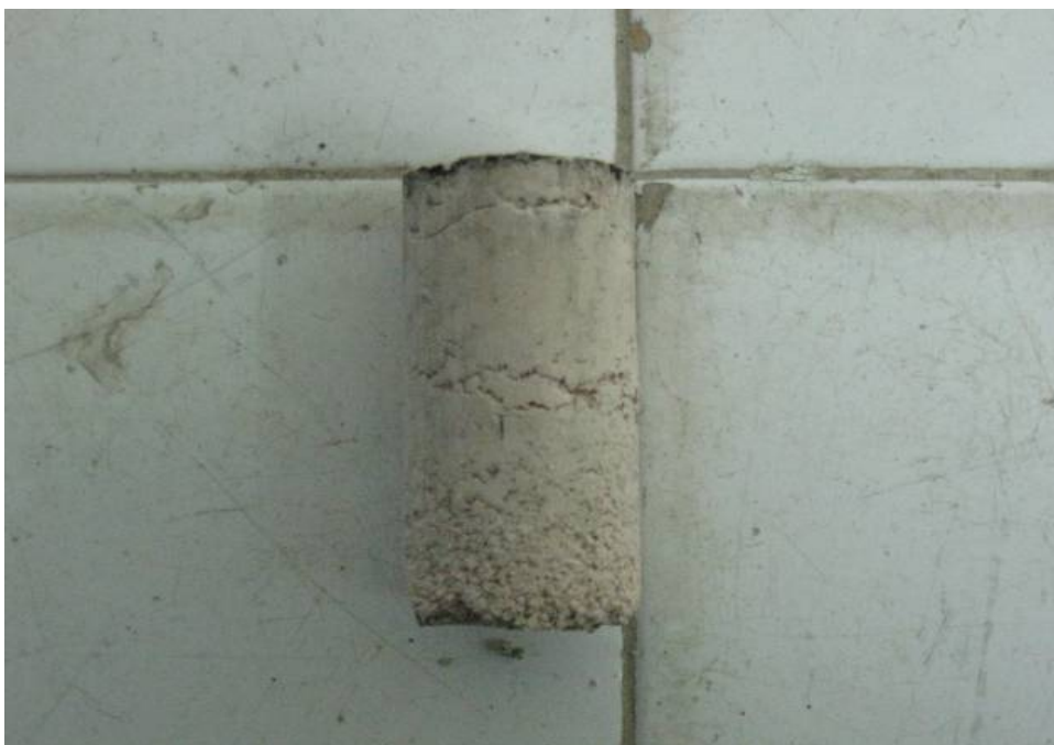
Figure 5.4. Bentonite and kaolinite mixture sample of size 3.3mm dia and 7.0mm height
