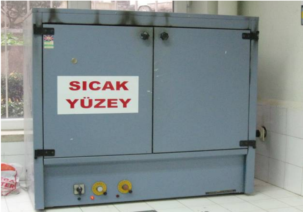
Figure 5.12. Oven inside the laboratory is used for drying soil samples
