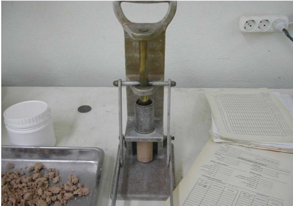
Figure 5.8. Special apparatus to take out specimens without breaking
