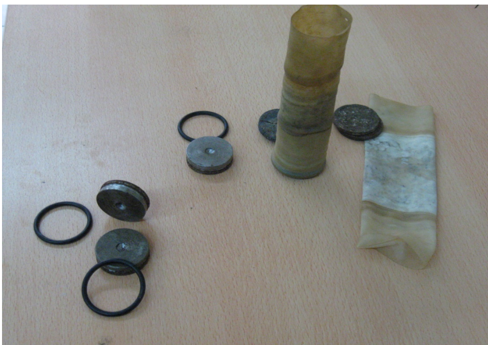
Figure 5.13. Metal caps are tightly fixed by rubber clamps from both ends of the flexible membrane before fitting in porous stones and the sample
