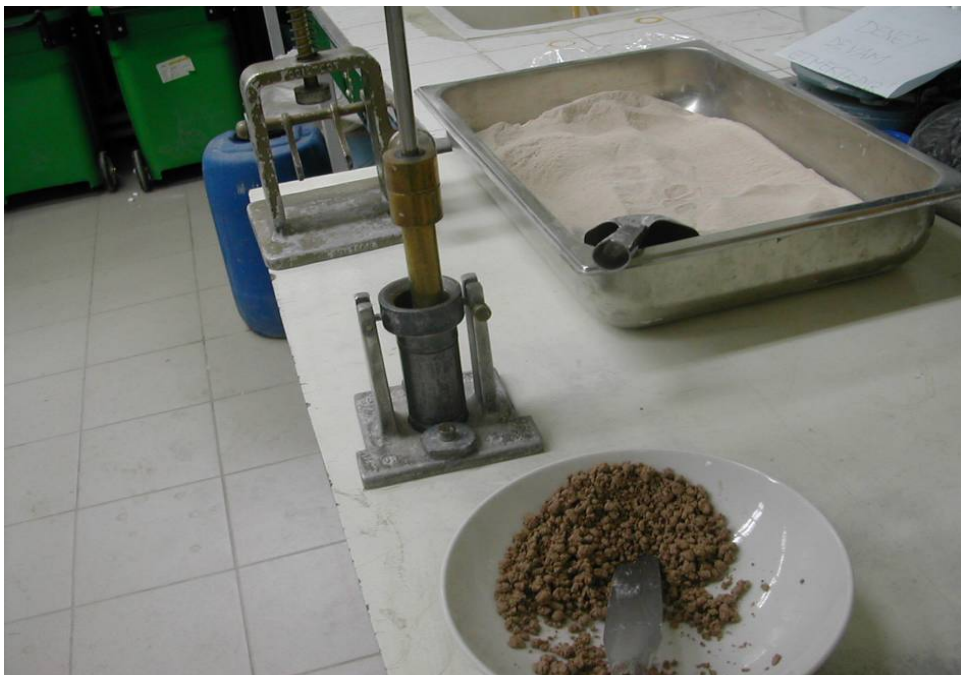
Figure 5.7. Harvard miniature compaction mold with 240gr weight hammer inside
