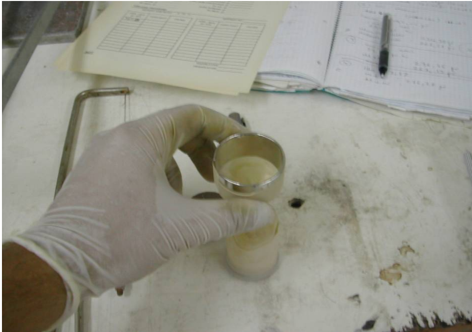
Figure 5.9. Flexible membrane used to wrap specimens
