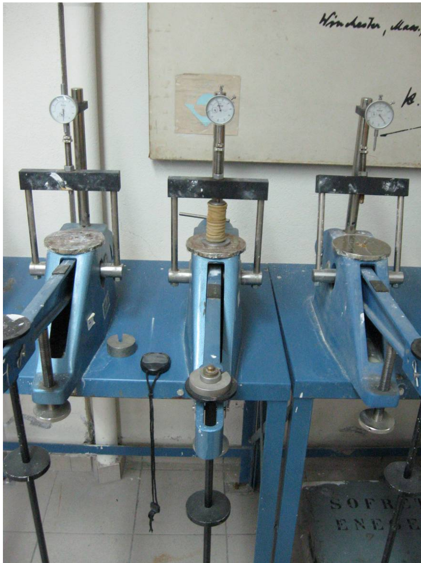
Figure 5.10. Oedometer EL25-0402 apparatus used for consolidation
