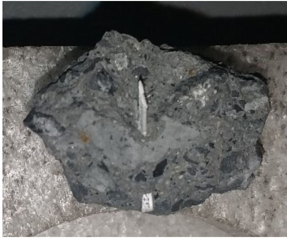
Figure 3.7. A test sample of fibrous-concrete for ESEM / EDAX analysis
