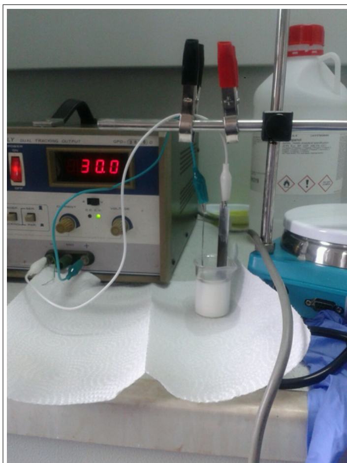
Figure 3.3 Experimental setup for EPD
