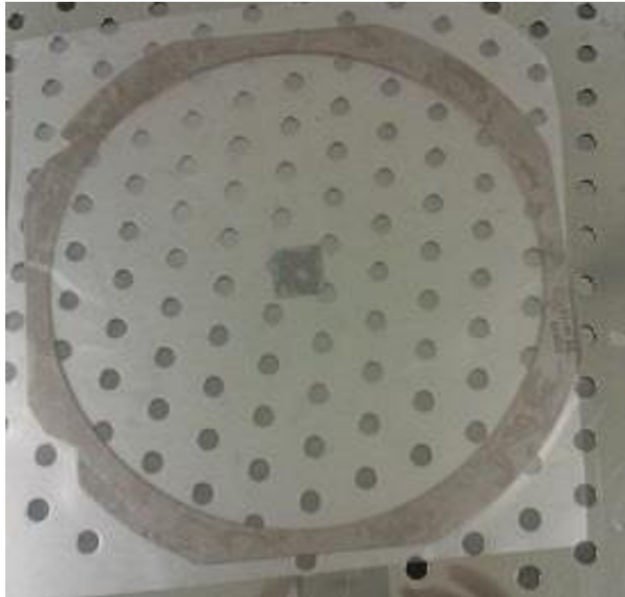
Figure 3.4. Wafer chip mounted on UV sensitive tape, ready to be diced
