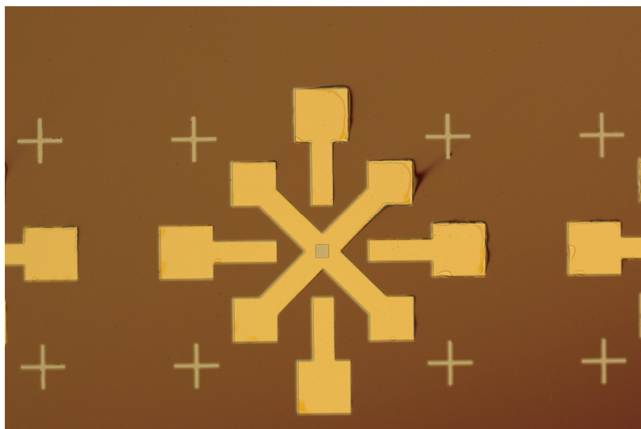
Figure A.6. Optical microscopy image after defining 30x30 \mu\text{m} device area
