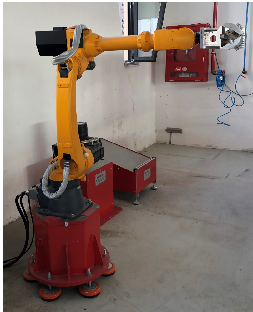
Figure 3.2. ESTUN ER16 industrial robot is used to implement the developed system. The robot is a six-axis articulated manipulator.
