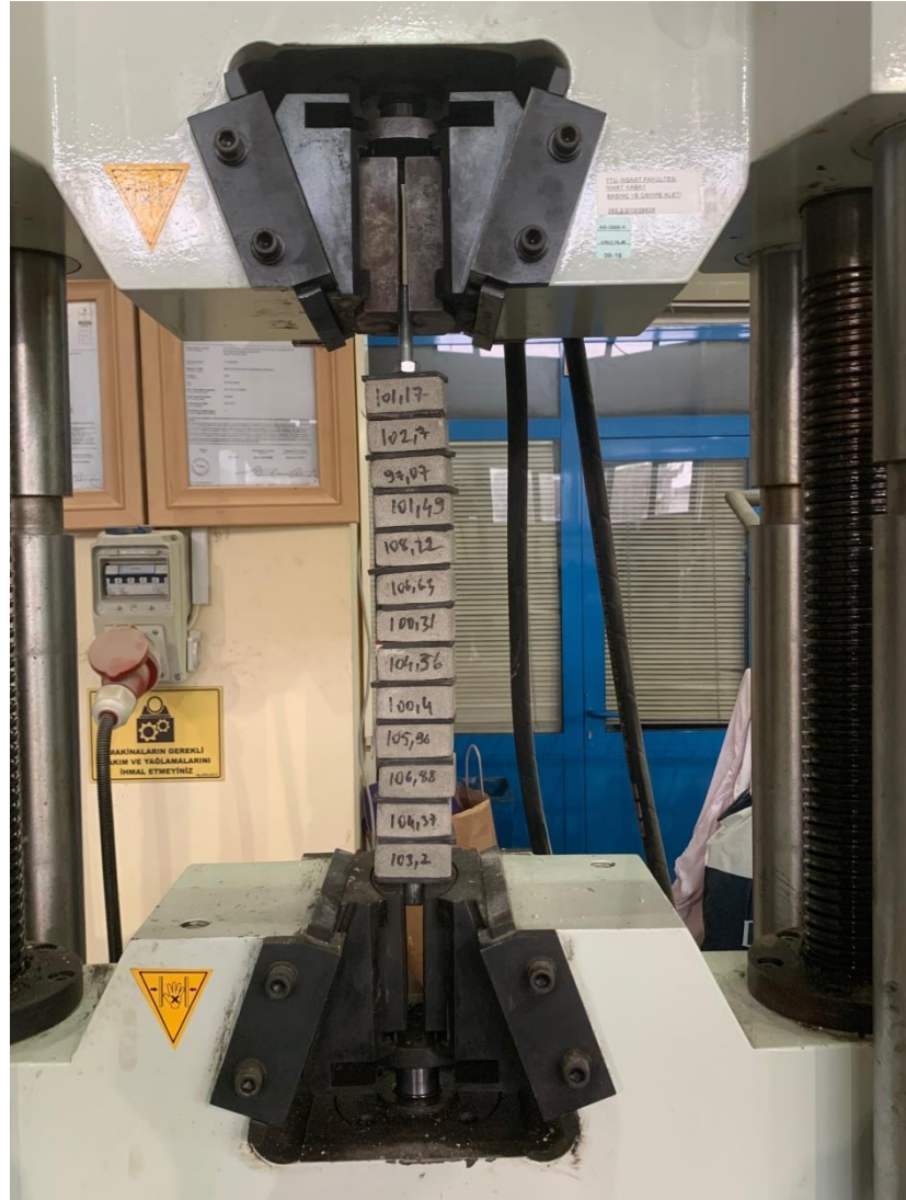
Figure 3.4. Steel Tension Test.
