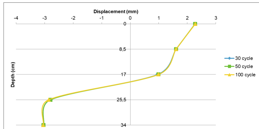
Figure 4.42. Displacement of the Segmental Pile with Post-Tension Force 2250 N in Medium-Dense Soil.
