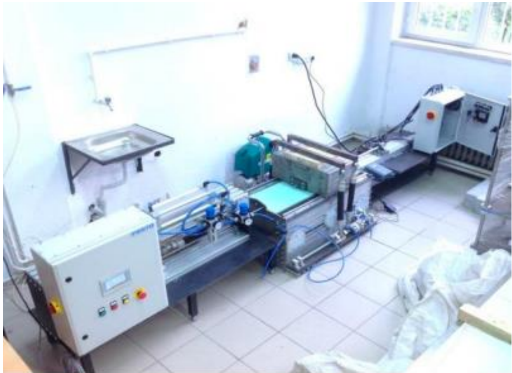
Figure 2.37. Large displacement constant contact area shear device [40].
