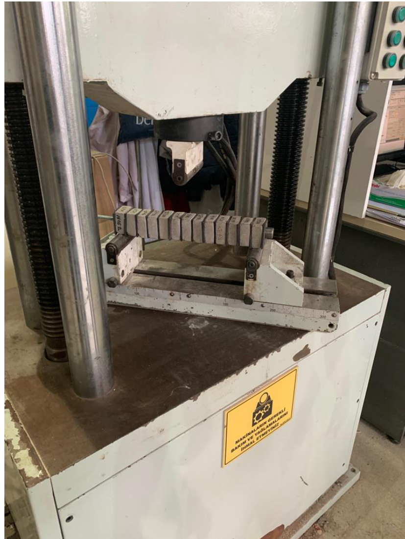
Figure 3.5. Three Point Bending Test.
