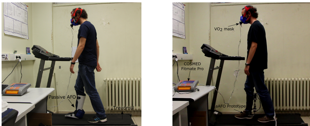
Figure 6.4. Cardiopulmonary exercise test. User wears a passive ankle-foot orthosis (left). User wears the active ankle-foot orthosis prototype (right).
