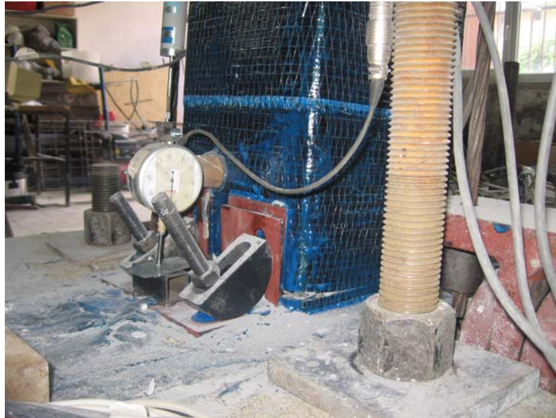
Figure 3.13. Rupture of CFRP in Specimen LS FRP
