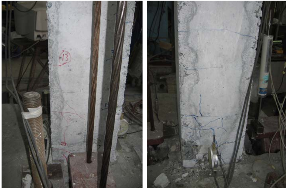
Figure 3.8. Column Cracks of Specimen LS
