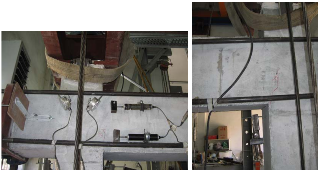
Figure 3.12. Beam Flexure Crack and Joint Crack of Specimen LS-FRP
