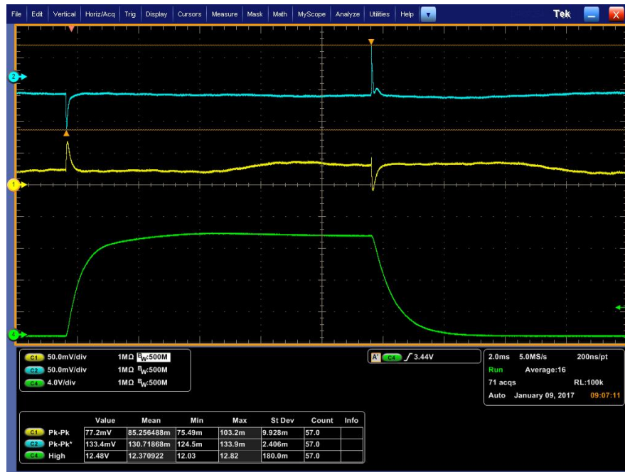
Figure 2.8. Beam current measurements. Green: Faraday cup, yellow and blue: ACCT signals. [5]
