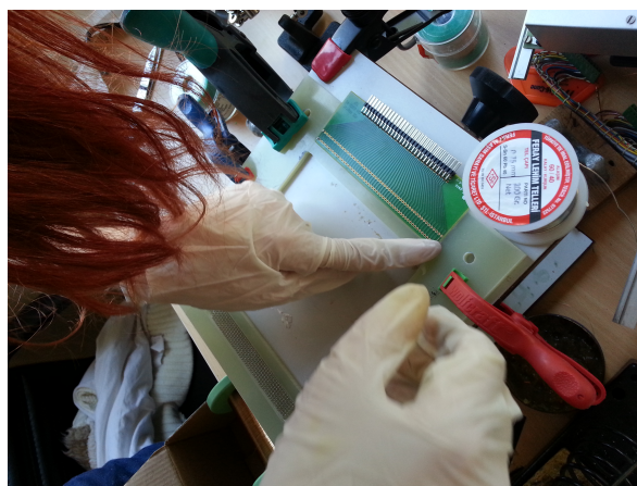
Figure 3.12. Stretching of the wires.
