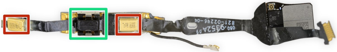
Figure 3.5. Onboard MEMS microphones, marked in red, in one of the disassembled earpiece to be used in voice and ambient noise pickup, adapted from [46].
