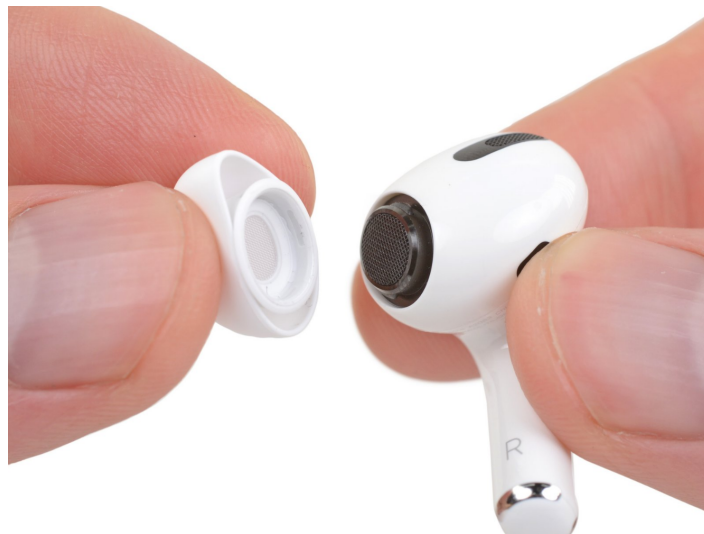
Figure 3.3. An Apple AirPods Pro true wireless headset piece with ear cover removed, adapted from [46].
