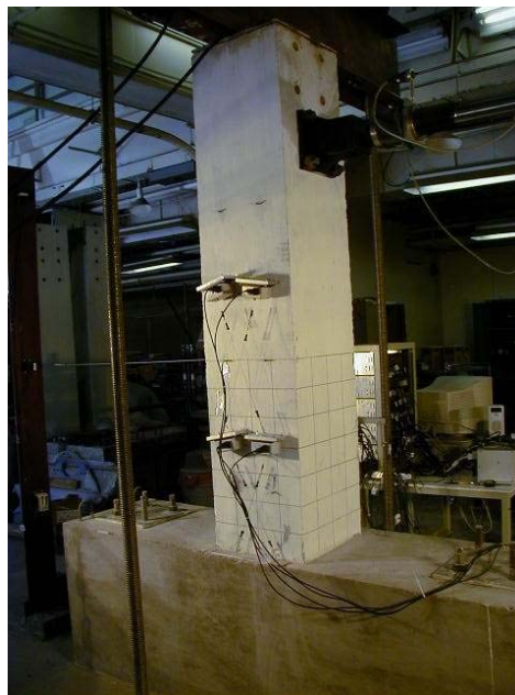
Figure 7.11. Shear Instrumentation (2S20H, 2S20HN, 2S30X, Melek, 2006).
