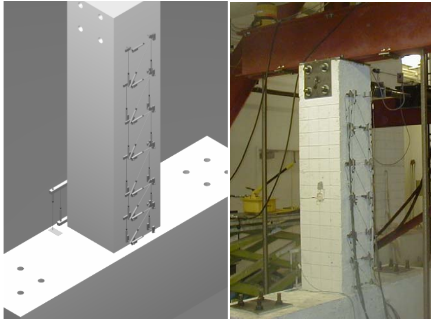
Figure 7.8. External Instrumentation Grid (2S10M, 2S20M, 2S30M, Melek, 2006).
