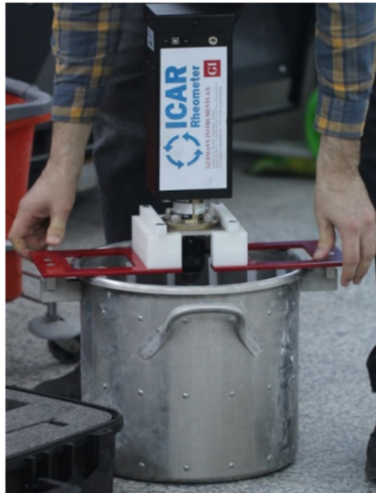
Figure 3.14. Rheology tests using a rheometer on SCC mixes.
