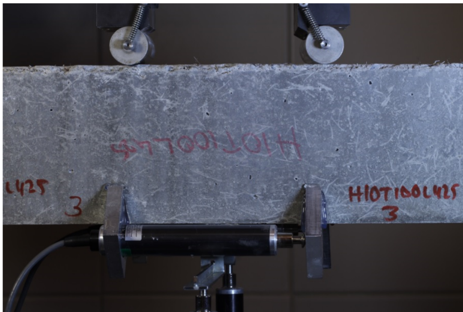
Figure 3.19. LVDT arrangement on a specimen.
