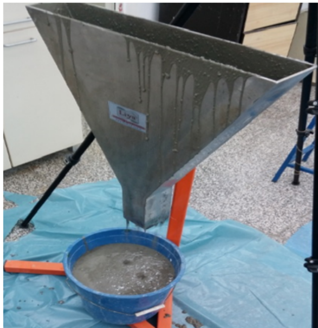
Figure 4.5. V-Funnel test - flowability of SCC specimens.
