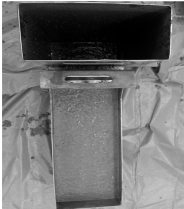
Figure 4.3. L-Box test - passing ability of SCC specimens.
