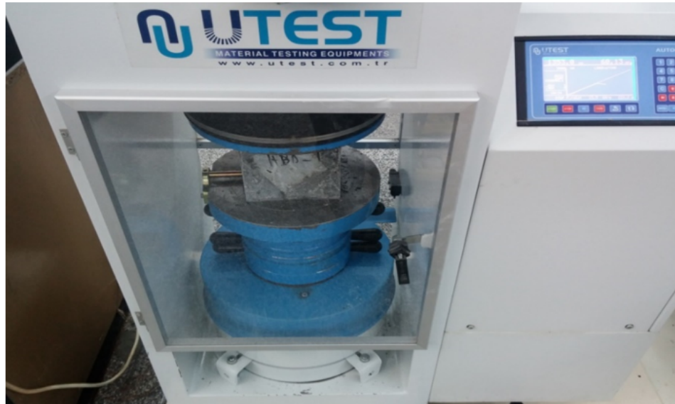
Figure 3.15. Compressive Strength Test.
