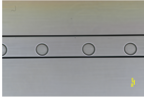
Figure 4.3. Oil phase 600 \mu\text{L/h} , aqueous phase 40 \mu\text{L/h} , droplet diameter 121.7 \mu\text{m} .
