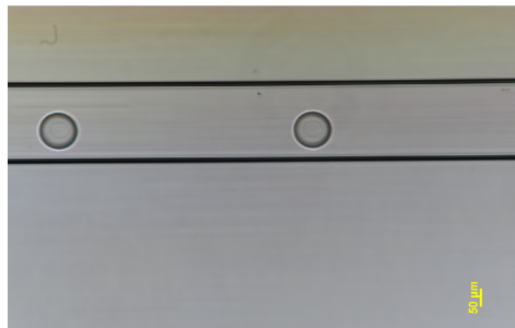
Figure 4.4. Oil phase 700 \mu\text{L/h} , aqueous phase 40 \mu\text{L/h} , droplet diameter 91 \mu\text{m} .
