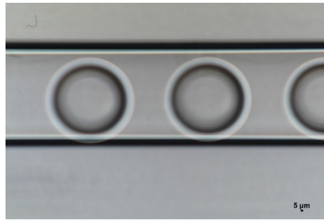
Figure 4.2. Oil phase 600 \mu\text{L}/\text{h} , aqueous phase 150 \mu\text{L}/\text{h} , droplet diameter 250 \mu\text{m} .
