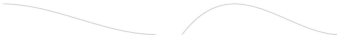
Figure 4.7. Two constraint modes for the left end of a beam that has attachment points at the two ends
